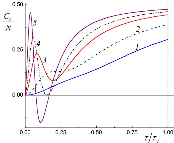
Figure 6: The isochoric heat capacity in the asymmetric phase for different values of the interaction constant: 1)  $|g| = 0.8$ ; 2)  $|g| = 0.66$ ; 3)  $|g| = 0.5$ ; 4)  $|g| = 0.425$ ; 5)  $|g| = 0.35$ .
