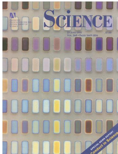
Figure 6: The June 23, 1995, cover of *Science*. A 128-member binary library fabricated by co-sputtering and mask technique.<sup>27</sup>
