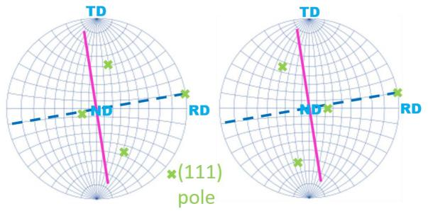
Supplementary fig. S3. (111) pole figures corresponding to the coherent  $\Sigma$ 3 twin boundary shown in supplementary Fig. S2b verifying its coherency.
