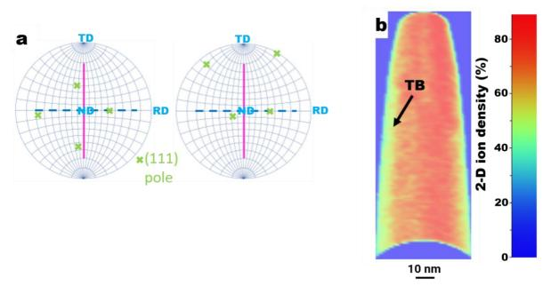
Supplementary fig. S5. Coherent  $\Sigma$ 3 twin boundary analyzed in Fig. 2. (a) (111) pole figures from the abutting grains verifying its coherency. (b) 2-D ion density (ion.%) composition plot indicating the studied twin boundary (TB).
