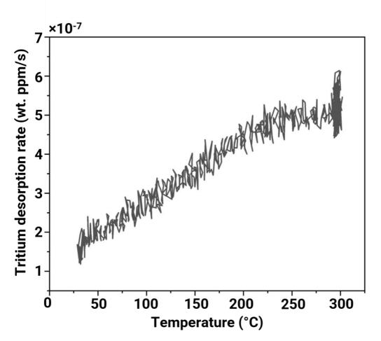
**Supplementary fig. S6. Thermal desorption analysis curve of the tritium-charged sample.** Tritium desorption rate calculated to wt. ppm/s is shown as a function of temperature (°C) from 30°C to 300°C.
