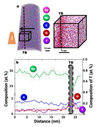
Fig. 3. (a) 3-D elemental map showing iron (Fe), manganese (Mn), carbon (C), oxygen (O) and tritium (T) atoms following the APT reconstruction. (b) Composition profile calculated with 1 nm bin width at the tritium-charged twin boundary (TB) highlighting the oxygen and tritium enrichment. Manganese depletion suggests that it is a coherent  $\Sigma$ 3 twin boundary.
