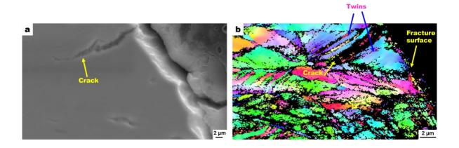
**Supplementary fig. S4. Fracture surface of the hydrogen-charged tensile specimen deformed to fracture.** (a) SEM image indicating a crack near the fracture surface. (b) Electron backscatter diffraction-inverse pole figure map with respect to normal direction (ND) out of the plane depicting twins near the crack.
