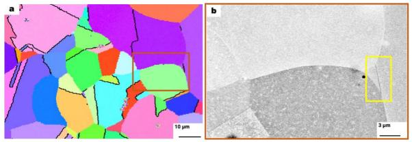
Supplementary fig. S2. Water-based corrosion of coherent twins. (a) EBSD-IPF map of the studied TWIP steel sample after performing the corrosion test highlighting the  $\Sigma 3$  twin boundaries in black. (b) A coherent  $\Sigma 3$  twin boundary indicated in yellow which is corroded. All EBSD-IPF maps are with respect to the normal direction out of the plane. ND – normal direction, TD – transverse direction, RD – rolling direction.
