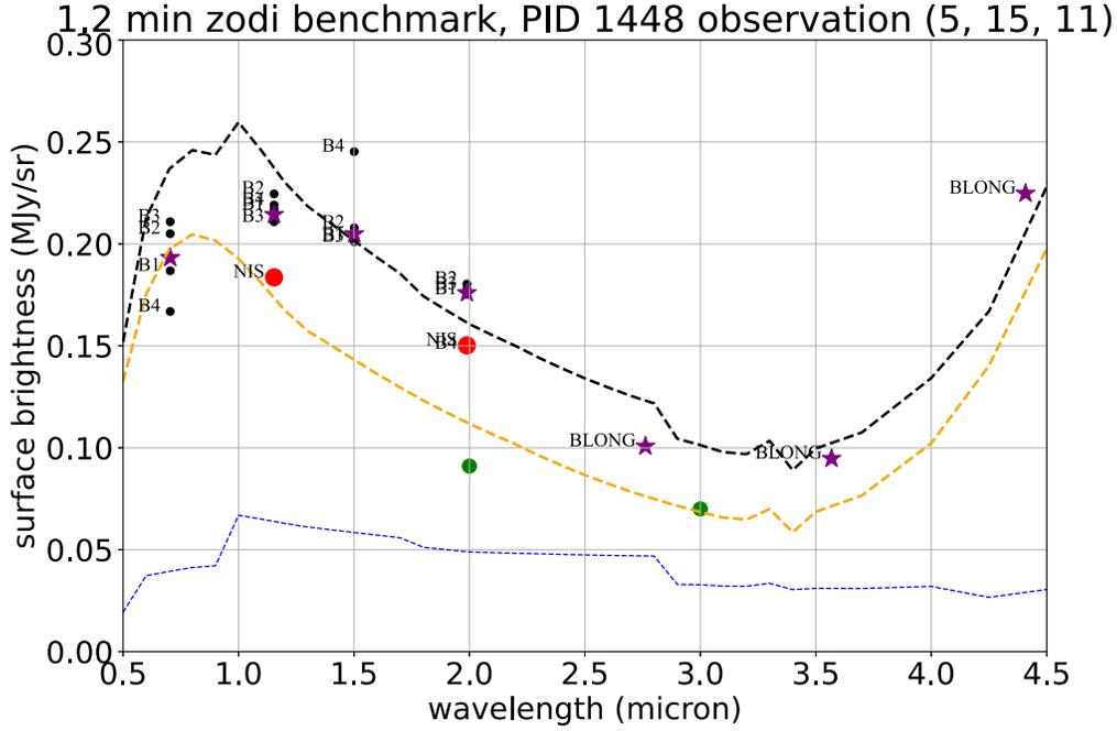
**Figure 5.** Backgrounds for the 1.2 minimum zodi benchmark pointing from commissioning observations. Symbols are the same as in Figure 4. Each detector is labeled (B1–B4 for the NIRCcam short-wavelength detectors in module B; BLONG for NIRCcam long-wavelength detector in module B, and NIS for the NIRISS detector). The chip-to-chip offsets are much larger than the statistical measurement uncertainties, indicating the importance of remaining systematic issues with calibration.
