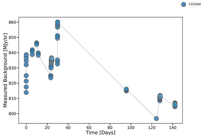
**Figure 8.** JWST background measurements at  $25.5 \mu\text{m}$ , spanning a period of about 145 days, starting in 2022 mid-March. Individual points represent the median across the MIRI imager field of view. The total range of the variation is 7%.
