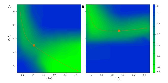
**Figure 2.** Interaction energies ( $E_{int}(r, R)$ ) for (A) an oxygen molecule and a Pt catalyst surface and (B) an oxygen molecule and a CuPt catalyst surface. The dotted orange line represents the trajectory of the oxygen molecule during the oxygen splitting reaction. The orange x marks the location of the activation barrier. Plots drawn using R and the akima package [34, 40]
