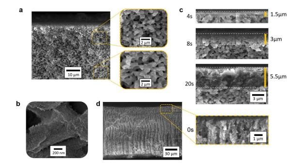
Figure 2. Cross-sectional scanning electron microscopy (SEM) micrographs of polymerized bijel films. A) VIPs-STRIPS bijel film. B) Jammed silica nanoparticle layer on the interface. C) The development of VIPS outer layer from the surface to the internal region with different evaporation time. D) Polymerized STRIPS bijel film from the same precursor mixture without VIPS treatment.
