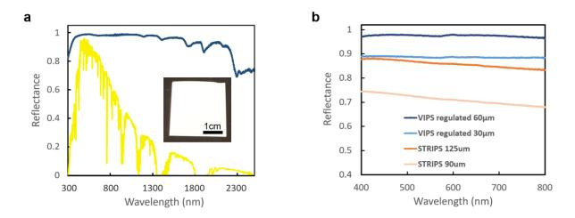
Figure 4. Spectral reflectance characterization. a) VIPS regulated bijels of ~ 130  $\mu$ m thickness. Yellow spectrum indicates normalized ASTM G173 Global solar spectrum. Inset shows macroscopic morphology of a ~ 130  $\mu$ m thick VIPS-STRIPS film. After polymerization, the dried sample forms a thick white opaque free-standing film. b) Regulated/non-regulated bijel films of different film thickness with incident angle of 45°.
