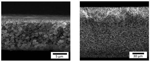
**Figure S1.** Cross-sectional SEM images of VIPS-STRIPS bijels film: (a) VIPS-STRIPS bijels with film thickness of around 10  $\mu$ m. (b) VIPS-STRIPS bijels with film thickness over 130  $\mu$ m.
