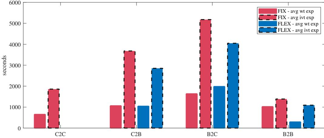
**Figure 9.** Final day average waiting time (weighted for denied boarding) and in-vehicle time (weighted for crowding) per passenger OD category (C2C, C2B, B2C, B2B) and per path type (FIX- for the C2C category, FIX-FLEX for C2B, FLEX-FIX for B2C, and FLEX- for B2B).
