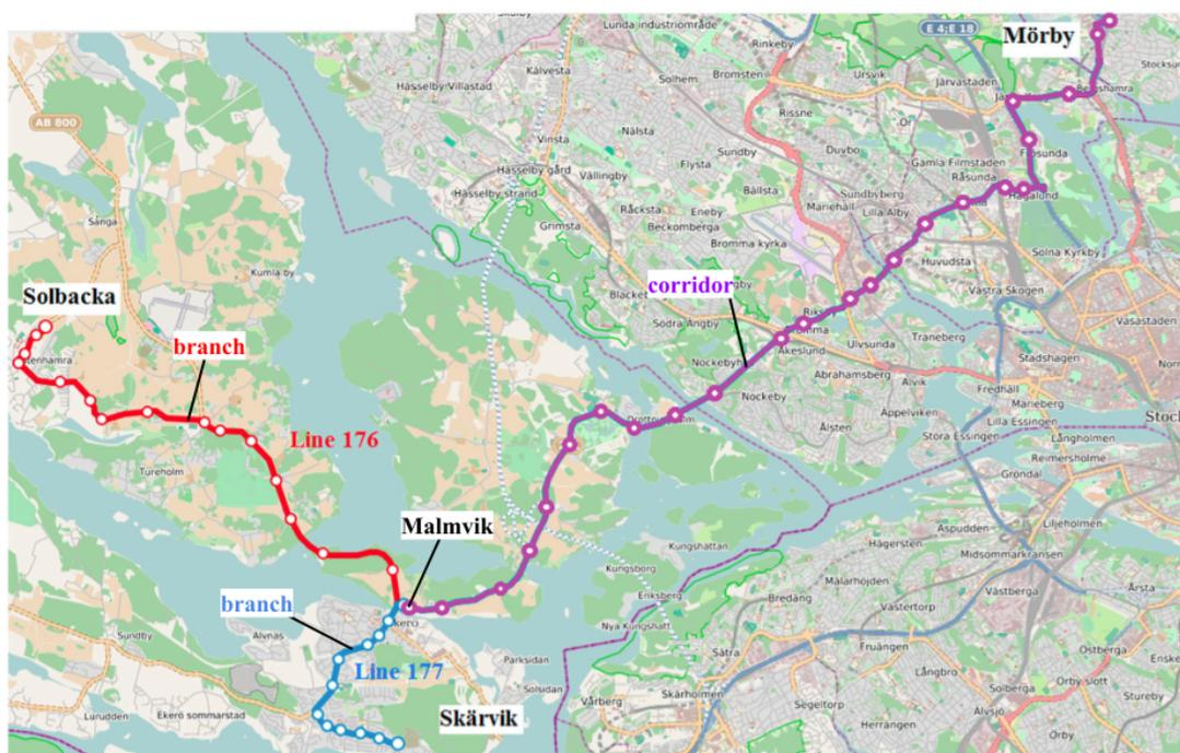
**Figure 7.** Lines 176 (red and purple segments) and 177 (blue and purple segment) in Stockholm. The purple segment is common for both lines. The lines merge/split at the stop Malmvik. Figure adapted from Laskaris et al. (2018), Figure 2.
