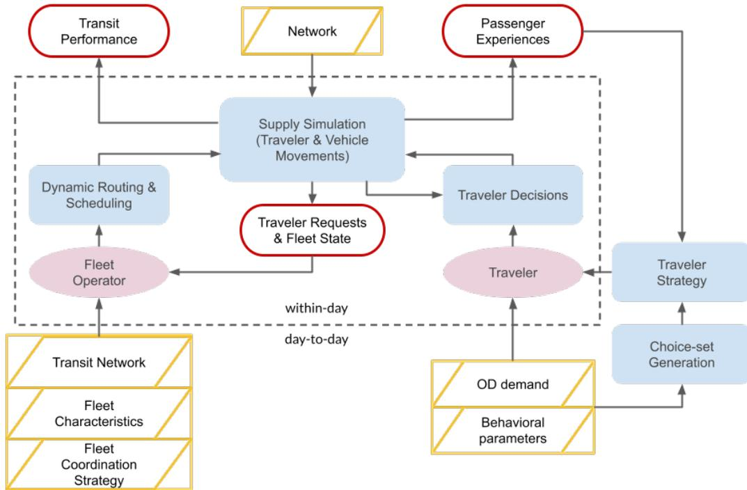
**Figure 1.** High-level overview of the simulation framework. Static inputs are marked with yellow boxes, key transit agents with purple ovals, processes with blue rectangles, and final and intermediate process outputs with red stadiums.
