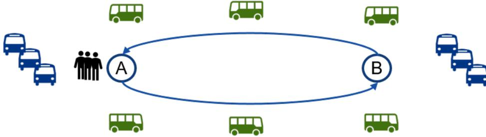
**Figure 5.** Two stop and two link network. Two services are available to travelers at stop A traveling to stop B: one fixed headway (10 min) service run with 100 passenger capacity buses (colored green), and one on-demand service run by 10 passenger capacity shuttles (colored blue). Both services use the same links with the same in-vehicle time (30 min) in either direction.
