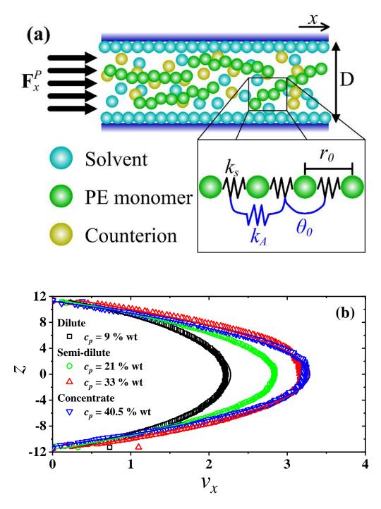
**Fig. 1**. (a) Illustration of the setup implemented in this work for confined PEs under a Poiseuille flow. A thin layer of solvent particles is formed close to the walls ( $z \le 0.15 r_c$ ), having a velocity equal to zero along the *z*-direction. The linear and angular bonding in PEs is depicted as well, wherein the constants  $k_s = 100$ ,  $r_0 = 0.7r_c$  (see eq. (1)) and  $\theta_0 = 180^\circ$
