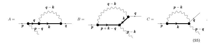
The crucial point is, that the imaginary part of the *A*- and *B*-blocks cancel each other out exactly. As a consequence, the lowest surviving order of the imaginary part of the self energy is Rayleigh-like Im $\Sigma \propto \sqrt{\lambda}p^4$ . To make the building-block structure appear in the equation for the renormalised vertex, we pull out a factor  $G_0^{-1}(\mathbf{k}, z)$  from the
