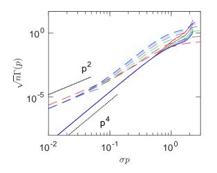
Figure 2. Sound attenuation as function of wavevector p. Rescaled data  $\sqrt{n}\Gamma(p)$  collapse for high densities n (see legend in Fig. 1) for small p. Solid lines follow from the imaginary part of the self-energy given by Eq. (4), dashed lines follow from planar diagrams [39] (see SI). The sound attenuation is calculated around the sound pole  $\omega = \sqrt{n\epsilon_0(p)}$ . Dotted lines represent asymptotic power laws.
