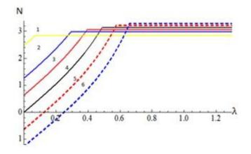
Fig.7 Dependences of the integral polarization of  $180^{\circ}$  DW on the parameter  $\lambda$  in the magnetic field H || Oy. The black line corresponds to p = 0, red - p = 0.1, blue - p = 0.2, yellow - p = 0.4, red dashed - p = -0.1, blue dashed - p = -0.2.
