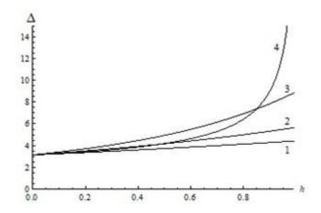
Fig.3 Dependences of the width of  $180^{\circ}$  DW  $\triangle$  on the magnetic field (**H**||Ox).Here  $\lambda = 0$ , line 1 corresponds to  $l_2 = 3$ ,  $2 - l_2 = 5$ ,  $3 - l_3 = 10$ ,  $4 - l_2 = 1000$ .
