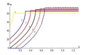
Fig.8 Dependences of the maximum angle of deviation from the homogeneous state  $\varphi_m$  180° DW on the parameter  $\lambda$  in the magnetic field H || Oy. The black line corresponds to p = 0, red - p = 0.1, blue - p = 0.2, yellow - p = 0.4, red dashed - p = -0.1, blue dashed - p = -0.2.
