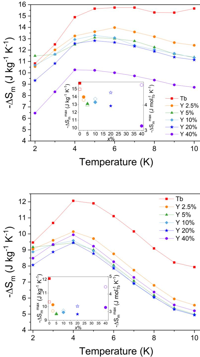
**Fig. 5:** Gravimetric magnetic entropy changes extracted from the magnetisation data for  $Tb_{1-x}Y_x(HCO_2)_3$  ( $x = 0, 0.025, 0.05, 0.10, 0.20, 0.40$ ) series for  $\Delta B = 5.0$  T (top) and  $\Delta B = 2.0$  T (bottom). Insets show the values of  $-\Delta S_m^{\max}$  in gravimetric (full symbols) and normalised molar (hollow symbols) units for each sample.
