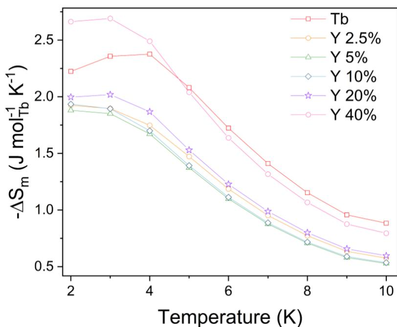
**Fig. S24:** Molar magnetic entropy changes, normalised per amount of Tb, extracted from the magnetisation data for  $\text{Tb}(\text{HCO}_2)_3$  and the  $\text{Tb}_{1-x}\text{Y}_x(\text{HCO}_2)_3$  ( $x = 0.025, 0.05, 0.10, 0.20, 0.40$ ) solid solutions for  $\Delta B = 1.0$  T.
