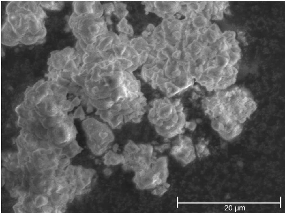
**Fig. S3:** SEM image of  $Y_{0.10}Tb_{0.90}(HCO_2)_3$  acquired with a secondary electron (SE) detector.
