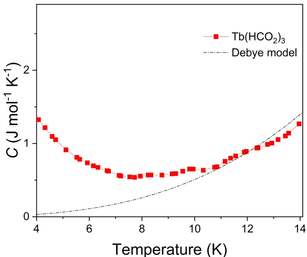
**Fig. S17:** Heat capacity data for  $\text{Tb}(\text{HCO}_2)_3$  between 4 to 14 K and Debye function plotted in the whole range of the plot, with the Debye temperature determined fitting the data between 8 to 14 K.
