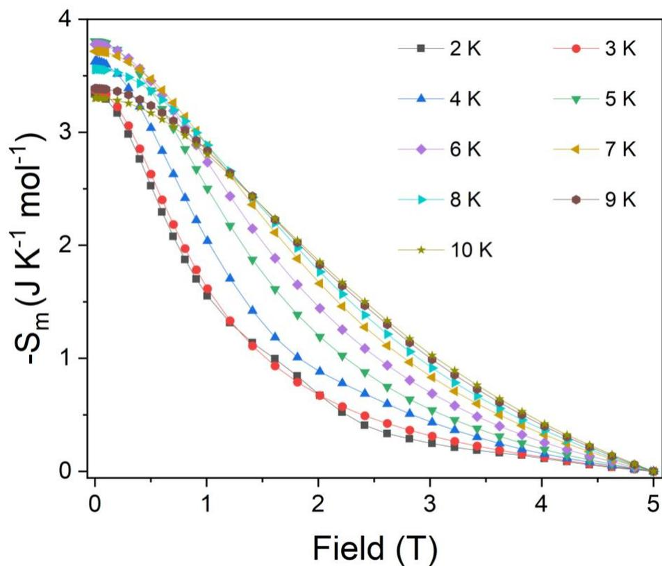
**Fig. S26:** Variation of magnetic entropy as a function of applied magnetic field extracted from the magnetisation data for  $\text{Tb}_{0.95}\text{Y}_{0.05}(\text{HCO}_2)_3$  at different temperatures.
