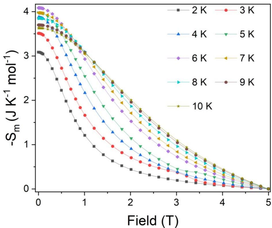
**Fig. S25:** Variation of magnetic entropy as a function of applied magnetic field extracted from the magnetisation data for  $\text{Tb}_{0.975}\text{Y}_{0.025}(\text{HCO}_2)_3$  at different temperatures.
