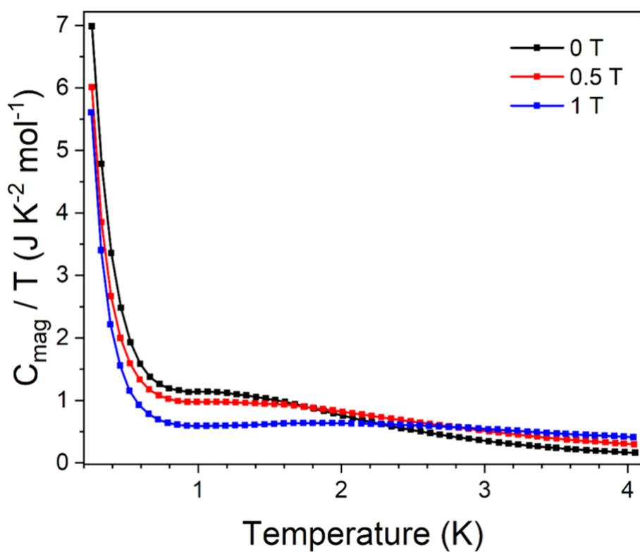
**Fig. S20:** Normalised magnetic heat capacity  $C_{\text{mag}}/T$  as a function of temperature  $T$  for  $\text{Y}_{0.40}\text{Tb}_{0.60}(\text{HCO}_2)_3$ .
