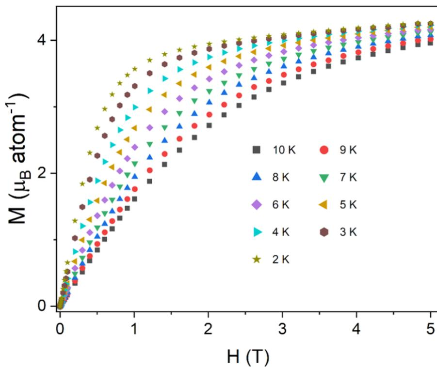
**Fig. S14:** Isothermal magnetisation measurements as a function of the applied magnetic field for  $Y_{0.10}Tb_{0.90}(HCO_2)_3$ .
