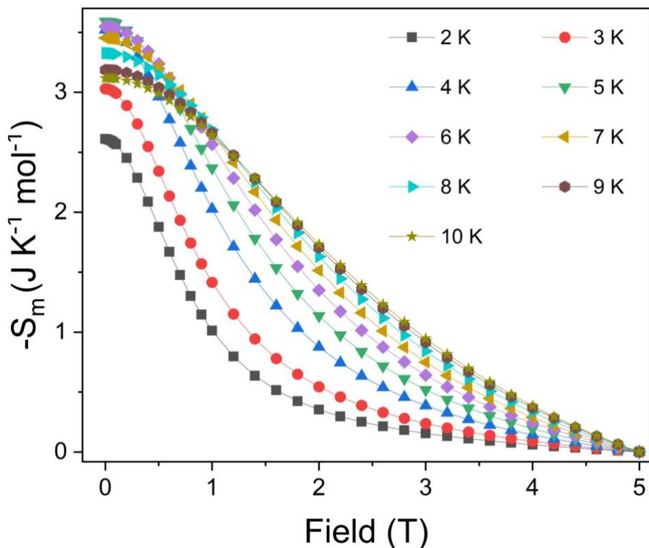
**Fig. S28:** Variation of magnetic entropy as a function of applied magnetic field extracted from the magnetisation data for  $\text{Tb}_{0.80}\text{Y}_{0.20}(\text{HCO}_2)_3$  at different temperatures.
