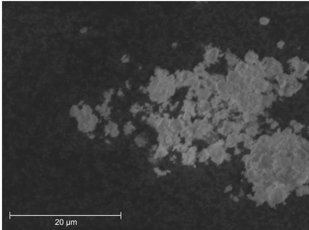
**Fig. S1:** SEM image of  $\text{Y}_{0.025}\text{Tb}_{0.975}(\text{HCO}_2)_3$  acquired with a secondary electron (SE) detector.
