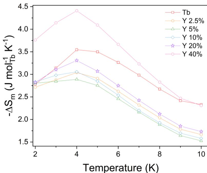
**Fig. S22:** Molar magnetic entropy changes, normalised per amount of Tb, extracted from the magnetisation data for  $\text{Tb}(\text{HCO}_2)_3$  and the  $\text{Tb}_{1-x}\text{Y}_x(\text{HCO}_2)_3$  ( $x = 0.025, 0.05, 0.10, 0.20, 0.40$ ) solid solutions for  $\Delta B = 2\text{-}0\text{T}$ .
