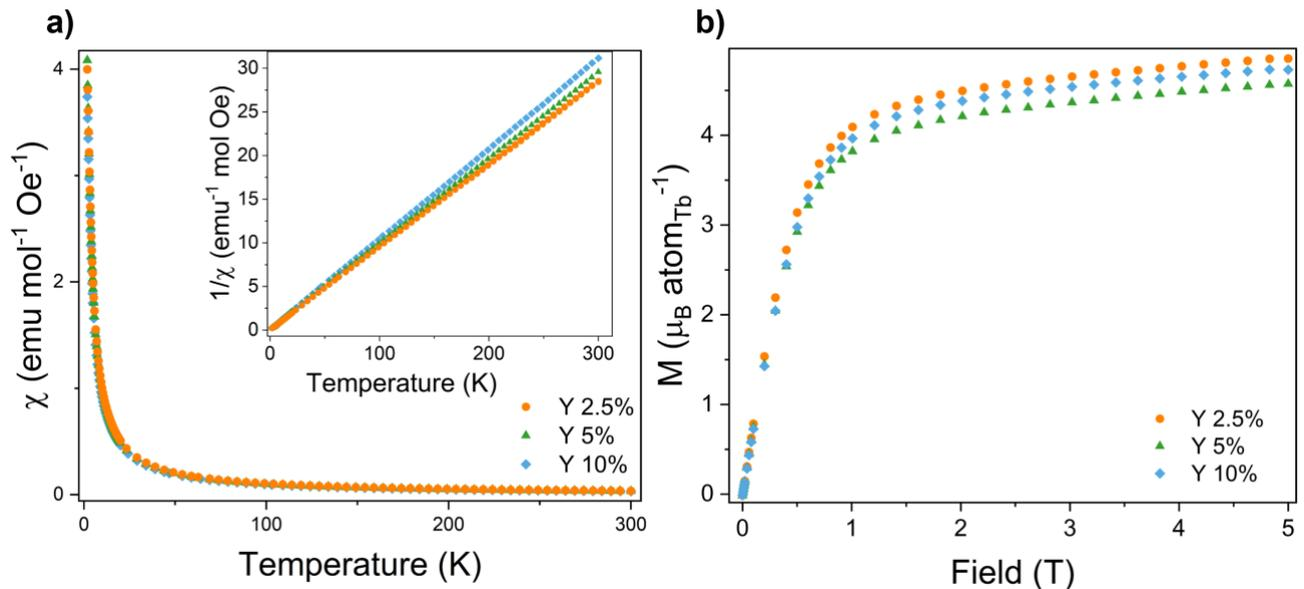
**Fig. 2:** a) FC molar susceptibility  $\chi(T)$  for  $\text{Tb}_{1-x}\text{Y}_x(\text{HCO}_2)_3$  with  $x = 0.025, 0.05, 0.10$ , measured from 2 – 300 K in a field of 0.1 T; the inverse molar susceptibility  $\chi^{-1}(T)$  is presented in the inset. b) Magnetisation plot of  $\text{Tb}_{1-x}\text{Y}_x(\text{HCO}_2)_3$  ( $x = 0.025, 0.05$  and 0.10) collected at 2 K for fields up to 5 T.
