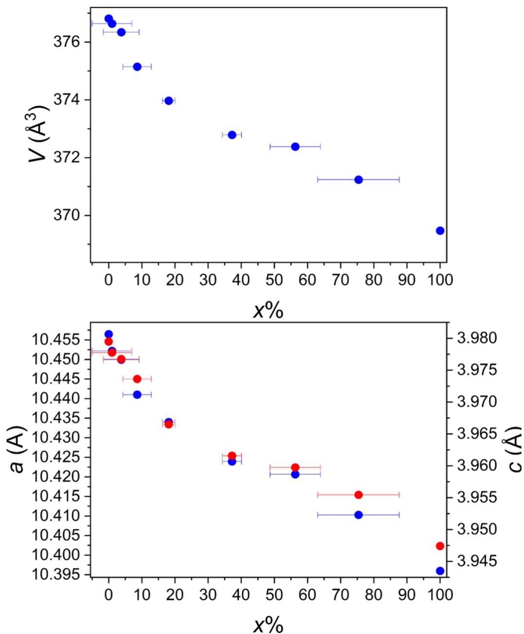
**Fig. S8** Plots of the unit cell volume (top) and lattice parameters  $a$  and  $c$  (bottom), the latter shown in blue and red, respectively, for the orthorhombic unit cell of  $Y_xTb_{1-x}(HCO_2)_3$ . Horizontal error bars show the uncertainty on the composition determined *via* X-ray fluorescence for the solid solutions.
