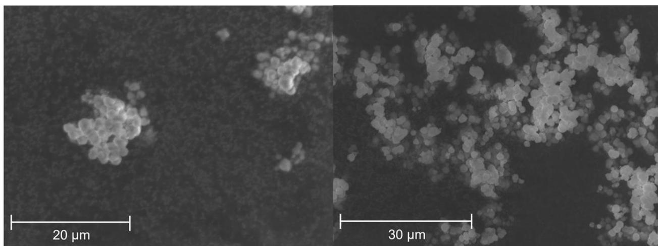
**Fig. S5:** SEM images of two different regions of  $Y_{0.40}Tb_{0.60}(HCO_2)_3$ , acquired with a secondary electron (SE) detector at different magnifications.
