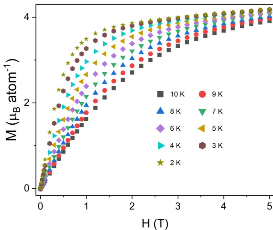
**Fig. S15:** Isothermal magnetisation measurements as a function of the applied magnetic field for  $Y_{0.20}Tb_{0.80}(HCO_2)_3$ .
