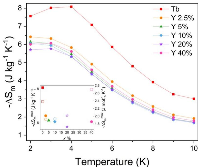
**Fig. S23:** Gravimetric magnetic entropy changes extracted from the magnetisation data for  $\text{Tb}(\text{HCO}_2)_3$  and the  $\text{Tb}_{1-x}\text{Y}_x(\text{HCO}_2)_3$  ( $x = 0.025, 0.05, 0.10, 0.20, 0.40$ ) solid solutions for  $\Delta B = 1.0$  T. The inset shows the values of  $-\Delta S_m^{\text{max}}$  in gravimetric (full symbols) and normalised molar (hollow symbols) units for each sample.
