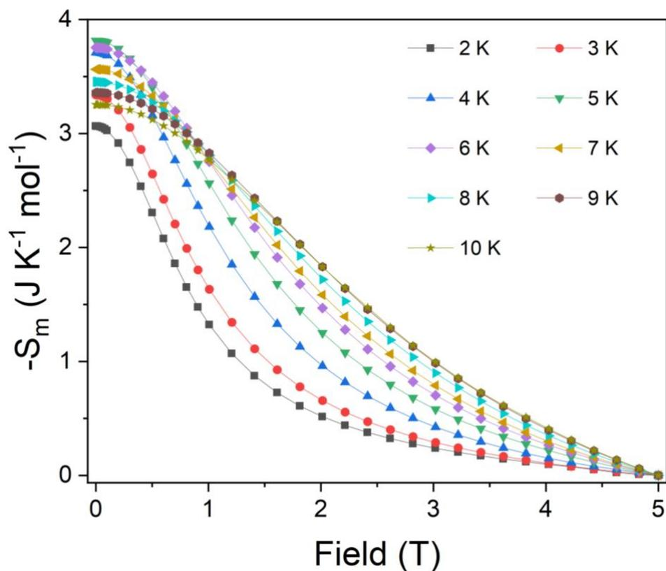
**Fig. S27:** Variation of magnetic entropy as a function of applied magnetic field extracted from the magnetisation data for  $\text{Tb}_{0.90}\text{Y}_{0.10}(\text{HCO}_2)_3$  at different temperatures.
