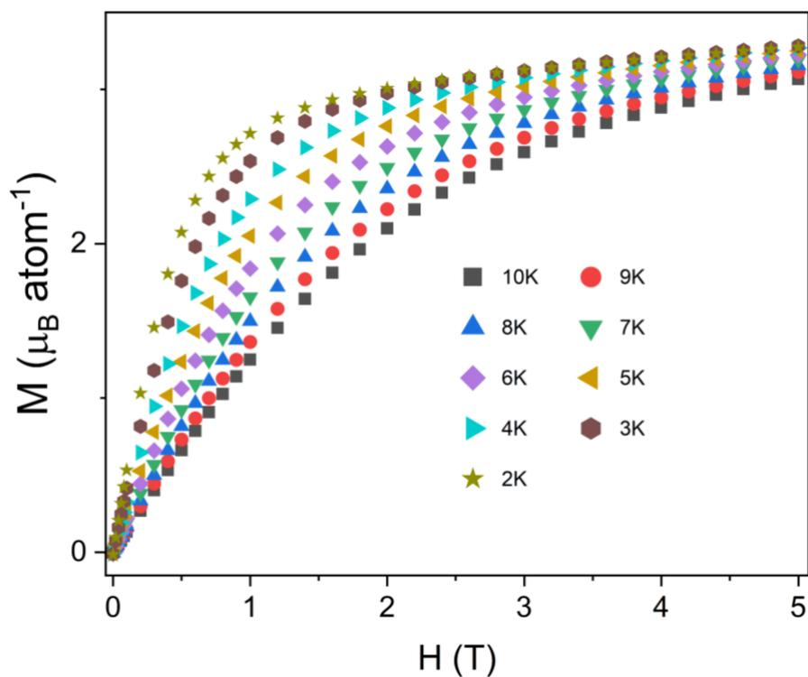
**Fig. S16:** Isothermal magnetisation measurements as a function of the applied magnetic field for  $\text{Y}_{0.40}\text{Tb}_{0.60}(\text{HCO}_2)_3$ .
