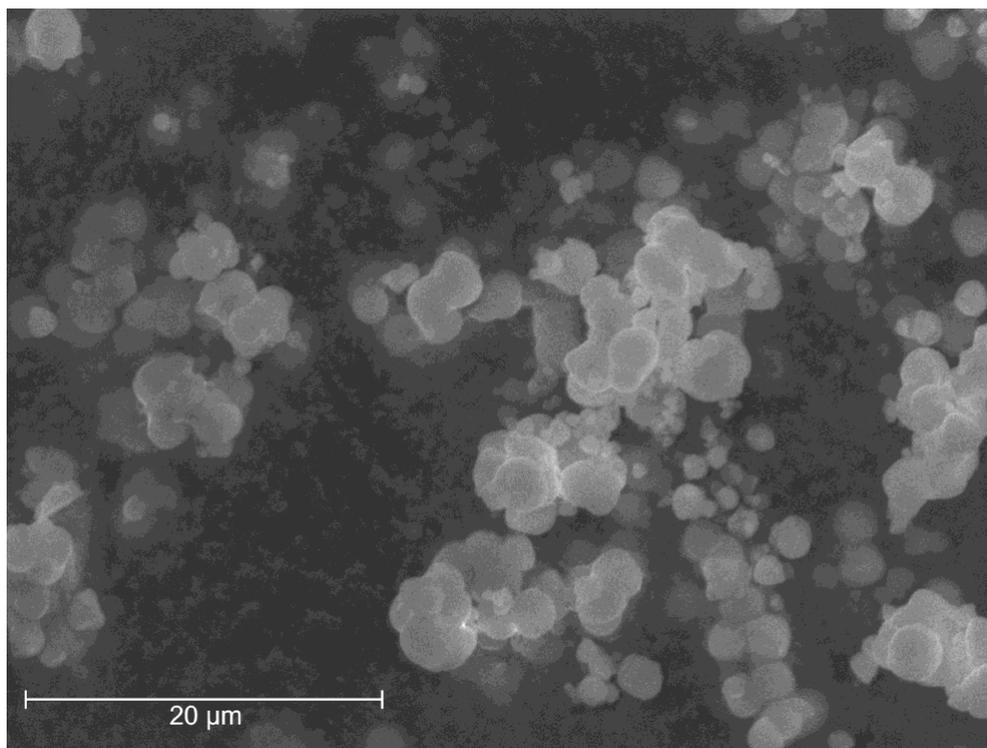
**Fig. S7:** SEM image of  $Y_{0.80}Tb_{0.20}(HCO_2)_3$ , acquired with a secondary electron (SE) detector.
