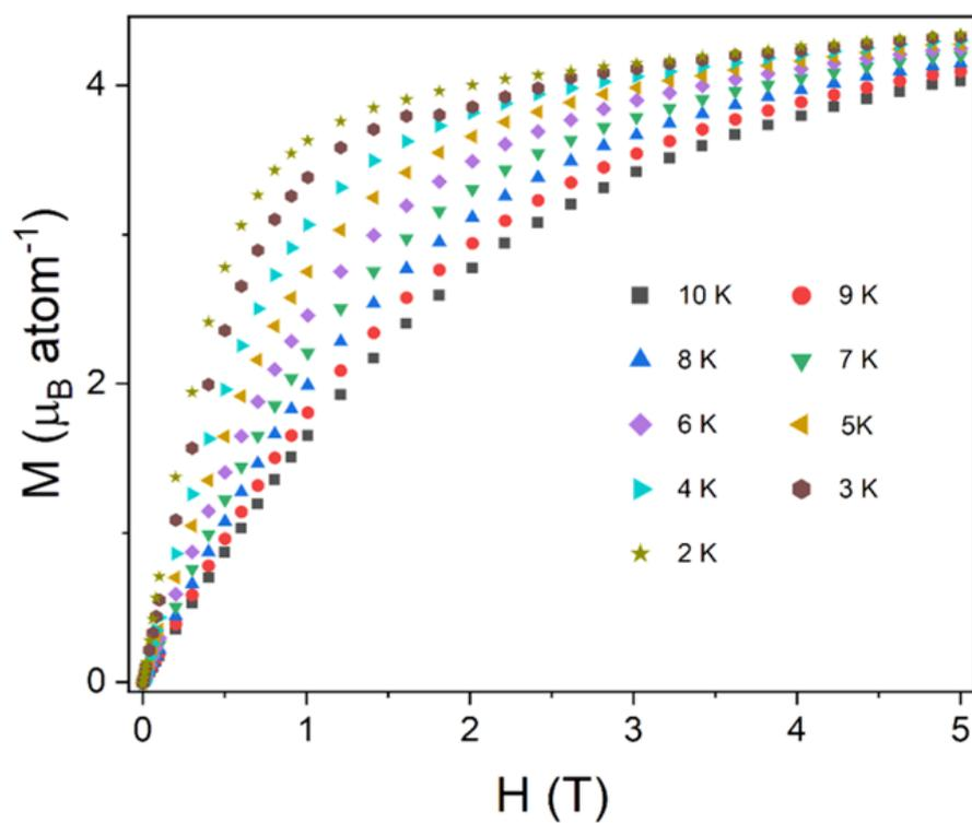
**Fig. S12:** Isothermal magnetisation measurements as a function of the applied magnetic field for  $\text{Y}_{0.025}\text{Tb}_{0.975}(\text{HCO}_2)_3$ .
