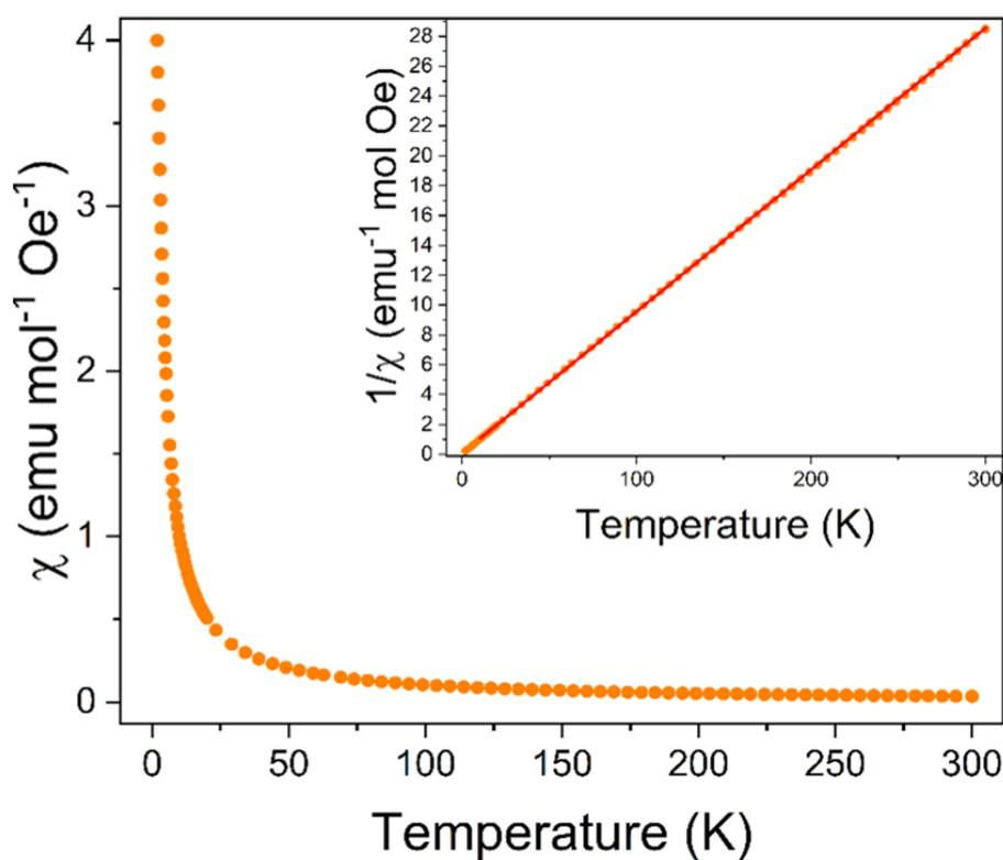
**Fig. S9:** FC susceptibility measurement for  $Y_{0.025}Tb_{0.975}(HCO_2)_3$  in a 0.1 T applied magnetic field. The insert shows the inverse susceptibility and the Curie-Weiss fit to the data obtained between 10 and 300 K.
