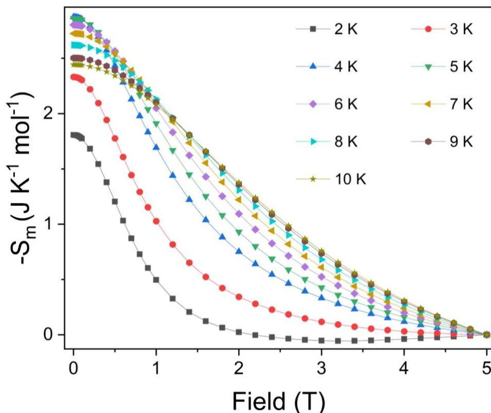
**Fig. S29:** Variation of magnetic entropy as a function of applied magnetic field extracted from the magnetisation data for  $\text{Tb}_{0.60}\text{Y}_{0.40}(\text{HCO}_2)_3$  at different temperatures.
