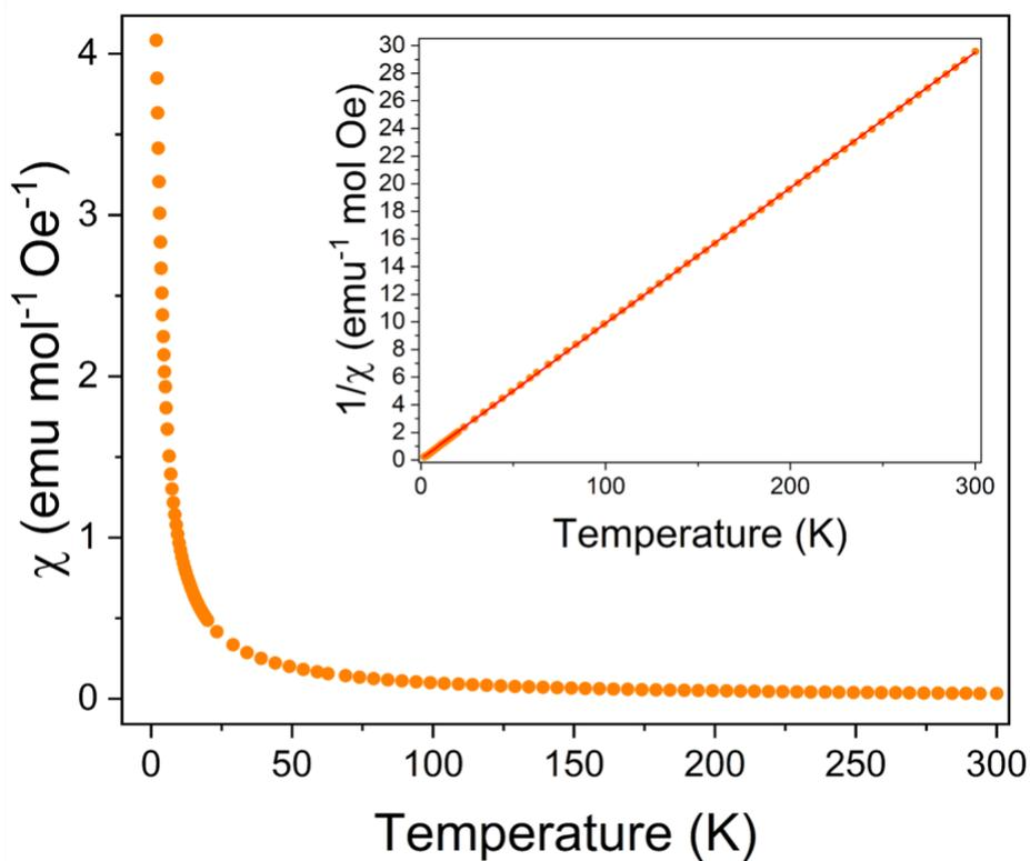
**Fig. S10:** FC susceptibility measurement for  $\text{Y}_{0.05}\text{Tb}_{0.95}(\text{HCO}_2)_3$  in a 0.1 T applied magnetic field. The insert shows the inverse susceptibility and the Curie-Weiss fit to the data obtained between 10 and 300 K.
