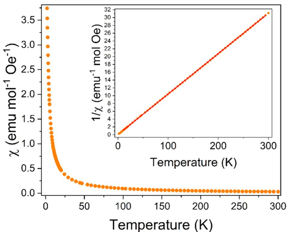
**Fig. S11:** FC susceptibility measurement for  $\text{Y}_{0.10}\text{Tb}_{0.90}(\text{HCO}_2)_3$  in a 0.1 T applied magnetic field. The insert shows the inverse susceptibility and the Curie-Weiss fit to the data obtained between 10 and 300 K.
