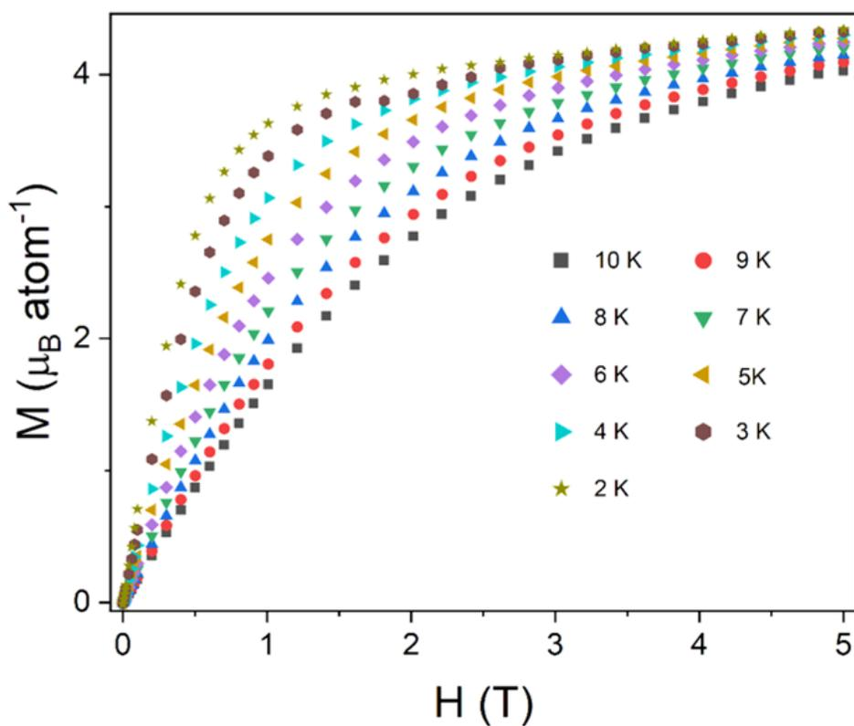
**Fig. S13:** Isothermal magnetisation measurements as a function of the applied magnetic field for  $\text{Y}_{0.05}\text{Tb}_{0.95}(\text{HCO}_2)_3$ .
