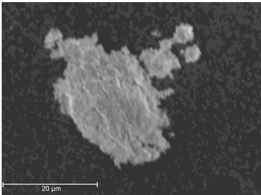
**Fig. S2:** SEM image of  $\text{Y}_{0.05}\text{Tb}_{0.95}(\text{HCO}_2)_3$  acquired with a secondary electron (SE) detector.
