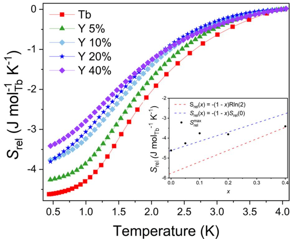
**Fig. 4:** Magnetic entropies per moles of Tb extracted from the heat capacity data for the  $\text{Tb}_{1-x}\text{Y}_x(\text{HCO}_2)_3$  ( $x = 0, 0.05, 0.10, 0.20, 0.40$ ) series in zero-field conditions. The inset shows the maximal values and the  $S_{\text{rel}}$  models derived from statistics.
