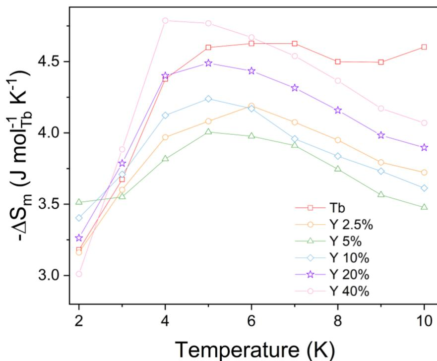
**Fig. S21:** Molar magnetic entropy changes, normalised per amount of Tb, extracted from the magnetisation data for  $\text{Tb}(\text{HCO}_2)_3$  and the  $\text{Tb}_{1-x}\text{Y}_x(\text{HCO}_2)_3$  ( $x = 0.025, 0.05, 0.10, 0.20, 0.40$ ) solid solutions for  $\Delta B = 5\text{-}0\text{T}$ .
