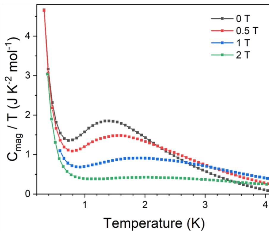
**Fig. S18:** Normalised magnetic heat capacity  $C_{\text{mag}}/T$  as a function of temperature  $T$  for  $\text{Y}_{0.10}\text{Tb}_{0.90}(\text{HCO}_2)_3$ .
