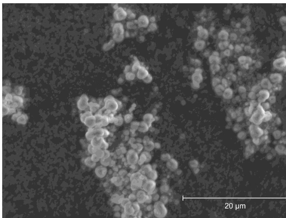
**Fig. S6:** SEM image of  $Y_{0.60}Tb_{0.40}(HCO_2)_3$ , acquired with a secondary electron (SE) detector.
