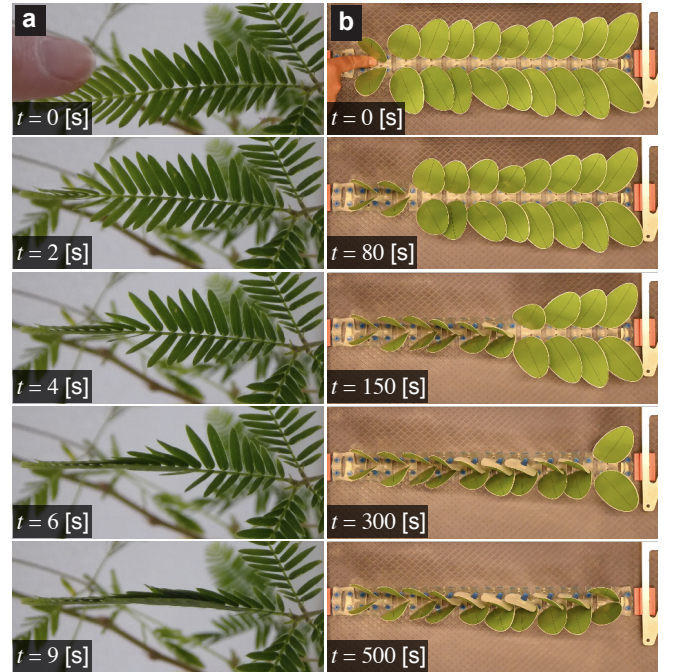
FIG. 1: Bio-mimicking slow kinks. (a) The leaflets of a Mimosa Pudica plant sense their environment by exhibiting a sequential folding process once touched. (b) A viscoelastic kirigami strip carrying paper leaflets shows a similar sequential folding after a touch..
