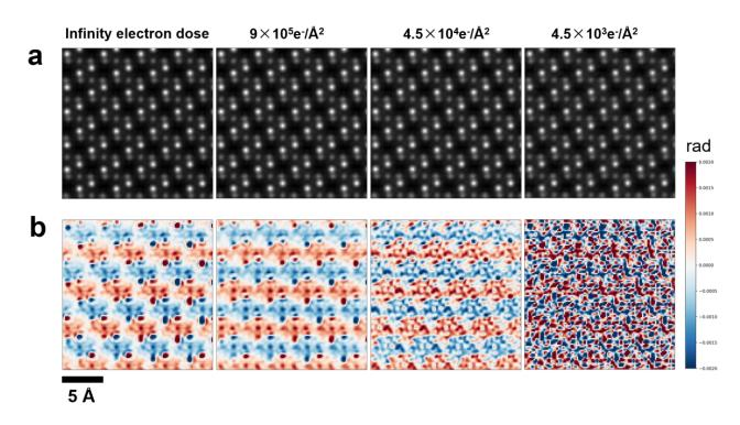
Fig. 3. The total and magnetic phases obtained with simulation datasets for different electron doses. a, the total phases via ptychographic reconstruction, b, the magnetic phases via Fourier separation. The sample thickness is 2.0 nm along,  $[11\overline{2}0]$  zone axis.
