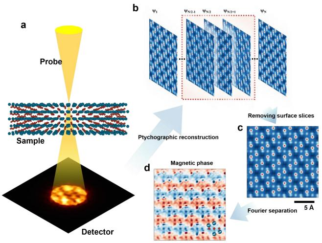
**Fig. 2. Workflow of extracting magnetic phase from total phase. a**, Experiment set up for electron ptychography; **b**, Reconstructed phase images of multiple slices; **c**, The averaged phase image of the central slices; **d**, The magnetic phase extracted by Fourier separation.
