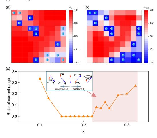
**Fig. 3.** Spatial distribution of (a)  $m_z$  and (b)  $H_{ex,z}$  in the sample with x = 0.15 and  $J_c = +5 \times 10^{11} \text{A/m}^2$ . The squares with blue balls represent Gd atoms and others represent FeCo atoms. (c) Ratio of current range as a function of x. The insert illustrates the phase diagram for  $x > x_{MC}$ .
