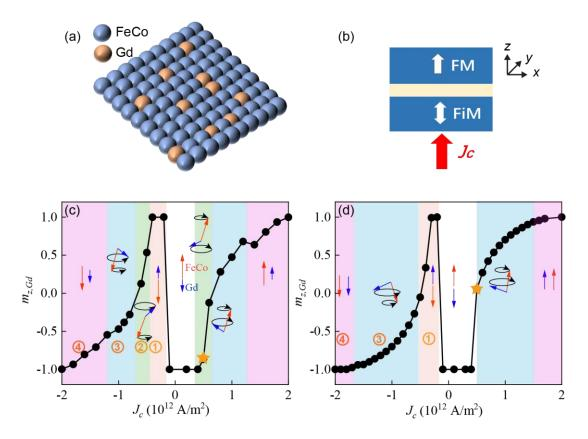
**Fig. 1.** Illustration of (a) the 2D atomistic model which consists of 100 atoms and (b) the device structure. Phase diagram of magnetization dynamics at (c) x = 0.1 and (d) x = 0.15. Red and blue arrows denote the magnetization direction of FeCo and Gd, respectively. m is calculated by averaging the atoms of the same type. The point marked with the star represents  $J_c = +5 \times 10^{11}$  A/m<sup>2</sup>.
