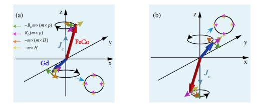
Fig. 2. Illustrations of the torques experienced by each atom when  $\mathbf{m}_{FeCo}$  and  $J_c$  are pointing in the (a)  $+\mathbf{z}$  and (b)  $-\mathbf{z}$  directions.
