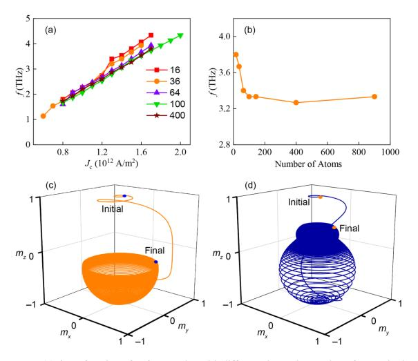
**Fig. 4.** (a) f as a function of  $J_c$  for samples with different sizes. The number of atoms is shown in the legend. (b) f as a function of sample size with  $J_c = 1.5 \times 10^{12} \text{ A/m}^2$ . The average oscillation trajectory of the sample with 16 atoms at (c)  $J_c = 1 \times 10^{12} \text{ A/m}^2$  and (d)  $J_c = 1.3 \times 10^{12} \text{ A/m}^2$ .
