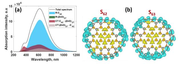
Figure 4. (a) Charge-transfer spectrum of the (ZnO)<sub>27</sub>C<sub>42</sub> including intrafragment electron redistribution (R) components and interfragment charge transfer (CT) contributions. (b) CDD for S<sub>62,63</sub> excited states in (ZnO)<sub>27</sub>C<sub>42</sub>. Yellow corresponds to positive charge distribution and cyan denotes negative charge distribution. Isosurface level is set to be 0.0002.
