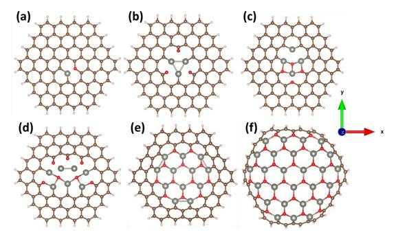
Figure 1. (Top view) Optimized structures of the (ZnO)<sub>n</sub>C<sub>96-2n</sub>: (a) n=1, (b) n=3, (c) n=4, (d) n=7, (e) n=12 and (f) n=27, respectively. Brown, whitish, blue, and red balls correspond to carbon, hydrogen, zinc, and oxygen atoms, respectively.
