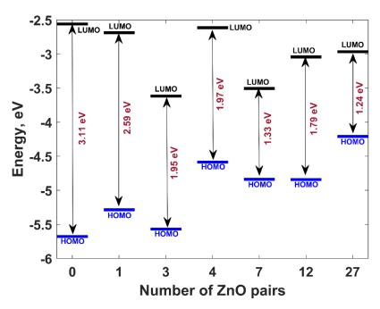
Figure S4. Molecular orbital diagram summarising all considered systems. The arrows designate HOMO–LUMO gaps.
