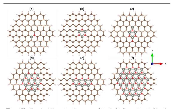
Figure S2. (Top view) Non-relaxed structures of the (ZnO)<sub>n</sub>C<sub>96-2n</sub>: (a) n=1, (b) n=3,
