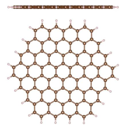
Figure S1. (Side and top views) Optimized structure of  $C_{96}H_{24}$  molecule. Brown and whitish balls correspond to carbon and hydrogen atoms, respectively.
