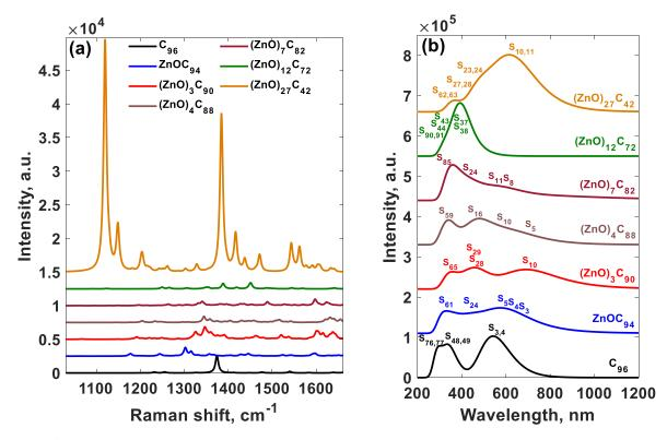
**Figure 2.** Predicted Raman spectra (a) and absorption spectra (b) of the  $(ZnO)_nC_{96-2n}$  structures, respectively.
