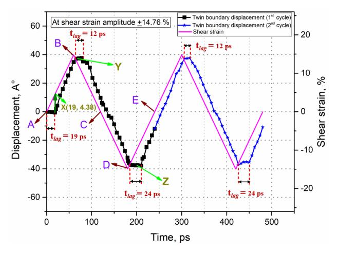
Fig. 4 Cyclic nature of twin boundary motion at 10 K for a shear strain amplitude of  $\pm 14.76\%$  and microstructures corresponding to the indicated locations A, B, C, D & E are shown in Fig. 2(A-E) respectively.
