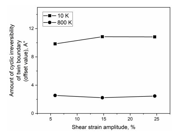
Fig. 5 Change in offset value after completion of a cycle with the applied cyclic shear strain amplitude at the temperatures 10 K and 800 K.
