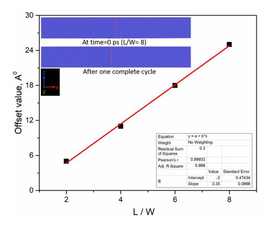
Fig. 14 Linear increase in offset value with increasing L/W ratio. Nanowires indicate the offset along with the absence of step formation once PBC is applied along Z-direction.
