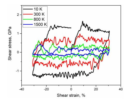
Fig. 11 Stress-strain hysteresis loops at different temperatures.
