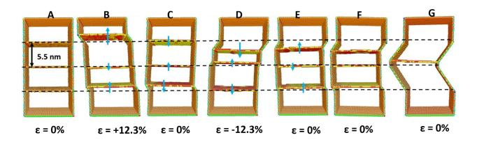
Fig. 12 Twin migration character in triple twin system. Green arrows indicate the migration or ready to migrate directions. Almost complete twin reversibility can be seen at C (for top twin), and at E (for middle and bottom twins). A-E indicate one complete cycle where F and G are deformed nanowires after completing the 10<sup>th</sup> and 50<sup>th</sup> cycles respectively.
