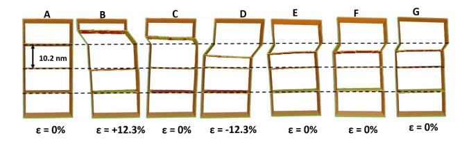
Fig. 13 Twin migration characters in the larger triple twin system. Only the top twin is migrating, whereas others are not. A-E indicate one complete cycle while F and G are deformed nanowires after completing the 10<sup>th</sup> and 50<sup>th</sup> cycles respectively.
