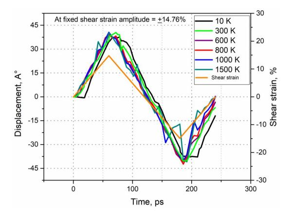
Fig. 6 Effect of temperature on twin boundary displacement concerning applied shear strain for the first cycle.
