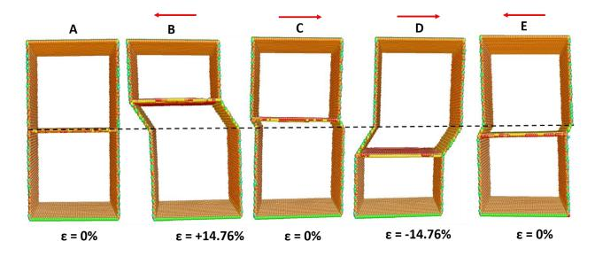
directions (Fig. 2 (B)- (E)). A low offset value indicates more recovered plasticity and vice versa. Thus, the twin boundary has an irreversible SCM character under cyclic shear loading.
