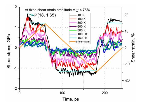
Fig. 9 Effect of temperature on the stress response of the system under applied cyclic shear strain amplitude of  $\pm 14.76\%$ . LT cyan colored lines on the 10K curve indicate the averaged TMS values. Only first cycle values have been shown for brevity.
