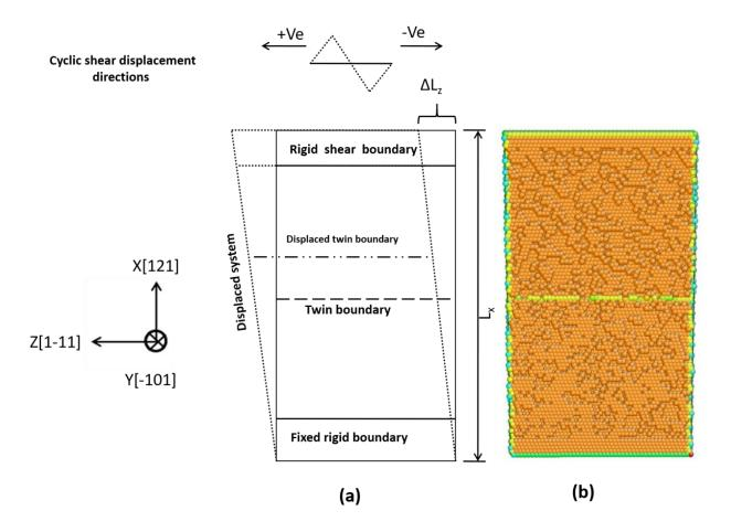
Fig. 1 (a) Schematic illustration of the model system under shear loading before shear displacement (solid lines) and after shear displacement (dotted lines). Twin boundary ( $\Sigma 3(112)$ ) displacement is marked by the dash-dot-dot line. (b) The equilibrated model system with twin boundary at the center.
