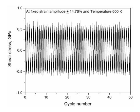
Fig. 16 Cyclic shear stress response of the system for the first 50 cycles at given shear strain amplitude of  $\pm 14.76\%$  and temperature at 600 K.
