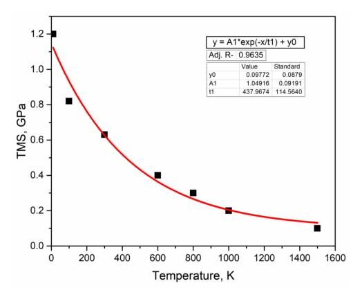
Fig. 10 An exponential decay nature of TMS value concerning temperature.
