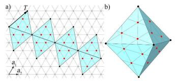
FIG. 3. Smooth mapping of the primitive hexagonal order onto the octahedron surface using the octahedron net. The case when the octahedron edge coincides with the translation T = (2,1) is illustrated. After the mapping, the nodes located on the octahedron faces (shown in red) have trivial symmetry, while the nodes located at the octahedron vertices have  $C_4$  symmetry.
