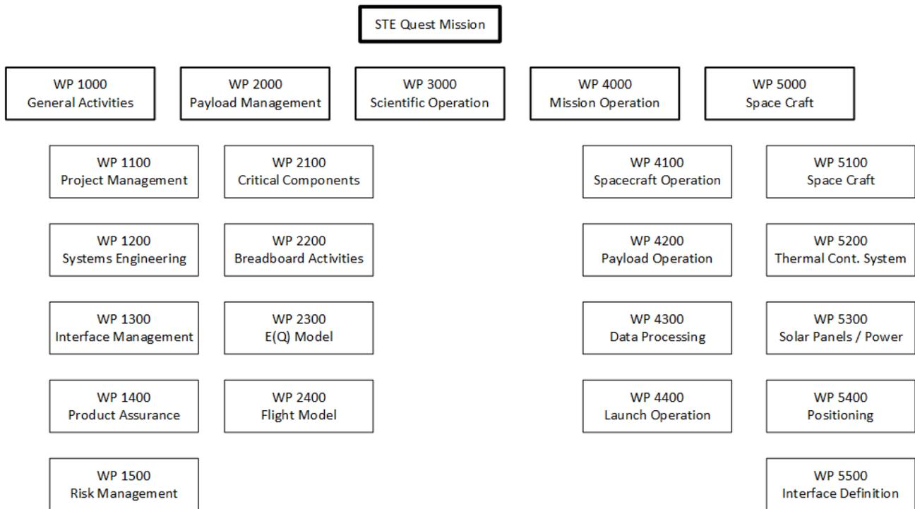
Figure 22: An overview over the work breakdown structure.
