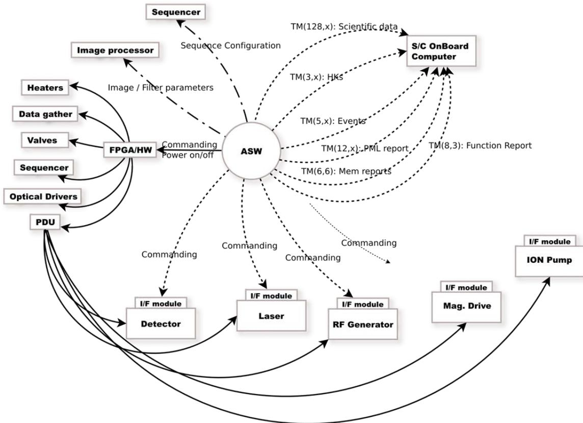
Figure 15: ATI software output context diagram (Application Software).
