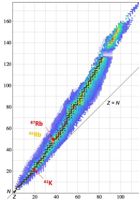
Figure 2: The valley of nuclei in the  $(N,Z)$  plane, with the  $^{85}\text{Rb}$ - $^{87}\text{Rb}$  combination from the M3 proposal in orange-red and the  $^{41}\text{K}$ - $^{87}\text{Rb}$  one from this STE-QUEST proposal in red.
