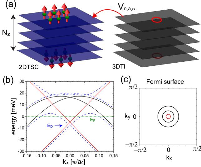
FIG. 1. (a) Schematic representation of the coupled 3DTI and 2DTSC systems with  $N_z$  layers. (b) Surface electronic structure: solid red and black lines represent the decoupled 3DTI and 2DTSC ( $V = 0$ ) systems, respectively, dashed lines the coupled ones ( $V \neq 0$ ). (c) Fermi surface of the coupled system. Parameters are  $(JS, \alpha, \mu, \mu_c) = (0, 0.1, 3.8, 0.06)t$ .
