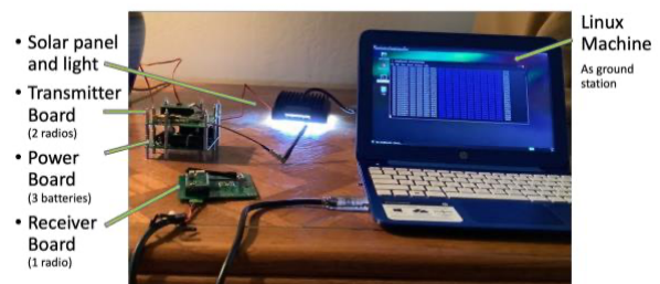
Figure 15: SSU's EdgeCube spacecraft bus, currently being tested as FlatSat by the 3UCubed students
