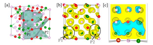
**Figure 4**. (a) 54-atom supercell for ternary NbTaV, (b) charge-density difference ( $\Delta \rho$  [LLD – no-LLD]), and (c) 2D project  $\Delta \rho$  on [100] plane showing charge activity at (P1, P2) in (b).
