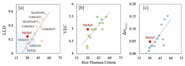
**Figure 3**. Comparison DFT-calculated Rice-Thomson criteria [53] with (a) LLD, (b) VEC, and (c)  $\Delta u_{x,y,z}$ . The ductile region is marked based on the criterion shown in Eq. (2).
