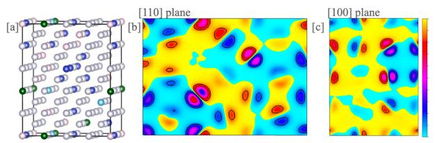
**Figure A5**. (a) Crystal structure of 120 atom quinary BCC Mo<sub>72</sub>W<sub>13</sub>Ta<sub>10</sub>Ti<sub>2.5</sub>Zr<sub>2.5</sub> MPEA, and increased charge activity along (b) (110), and (c) (100) planes.
