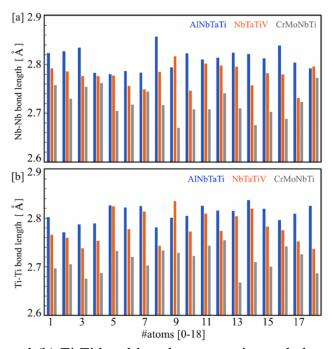
Figure A1. (a) Nb-Nb, and (b) Ti-Ti bond-length compression and elongation in (a) AlNbTaTi,(b) NbTaTiV, and (c) CrMoNbTi due to change in chemical environment in RMPEAs.In Fig. A2, we also show the bond-length distribution of selected RMPEAs, where AlNbTaTi with
