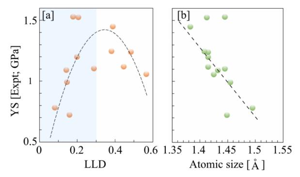
**Figure A4**. Measured yield strength (GPa) for bcc MPEAs vs. LLD (a) and atomic size (b). Higher ductility connects with a lower strength (see **Fig. 2**), shaded area in (a). MPEA strength decreases with increasing average atomic size (b).
