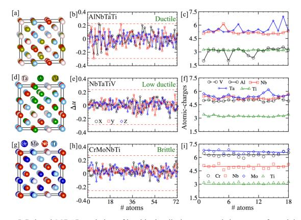
**Figure 5.** Relaxed SCRAPs and plots of local lattice displacement and charge-transfer activity in (a-c) AlNbTaTi (high ductility), (d-f) NbTaTiV (low ductility), and (g-i) CrMoNbTi (no ductility).
