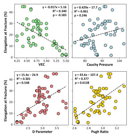
Figure 1. Linear models, coefficient of determination, and Pearson correlation between compressive fracture strain of 56 RMPEAs (see more detail in Table A1) and the following ductility indicators: VEC, Cauchy pressure, Pugh ratio, and the Rice criterion.
