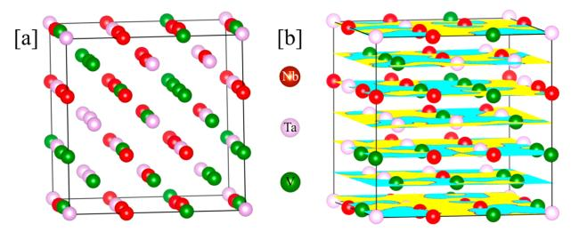
**Figure A3**. (a) A 54-atom supercell of fully relaxed ternary bcc NbTaV. (b) 2D projected charge density difference calculated at same lattice constants for fully relaxed vs. non-relaxed supercells.
