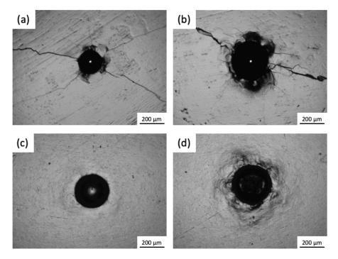
**Figure 7**. Optical images around Rockwell indents showing crack formations on (a,b) NbTaMoW (LLD=0.566) but not on (c,d)  $Mo_{72}W_{13}Ta_{10}Ti_{2.5}Zr_{2.5}$  (LLD=0.255). This suggests improved ductility for  $Mo_{72}W_{13}Ta_{10}Ti_{2.5}Zr_{2.5}$ , as predicted by LLD metric in **Table 4**. The indents are made using Rockwell hardness testers with 60 kgf (a,c) and 150 kgf (b,d) load, respectively.
