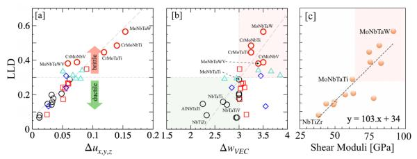
**Figure 2**. LLD metric versus (a) magnitude of vector atomic displacement from the average lattice  $\Delta u_{x,y,z}$ , and (b)  $\Delta w_{VEC}$  [regions: ductile (green) and brittle (red)], and (c) shear moduli (GPa). Ductile behavior of 17 RMPEAs designed in our ULTIMATE program [65] was also assessed: (red squares; 9), ( blue diamonds; 3), and ( cyan triangles; 5).
