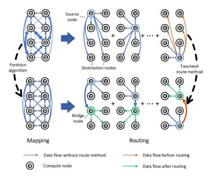
fig. S2 Illustration of the partition algorithm and routing method.
