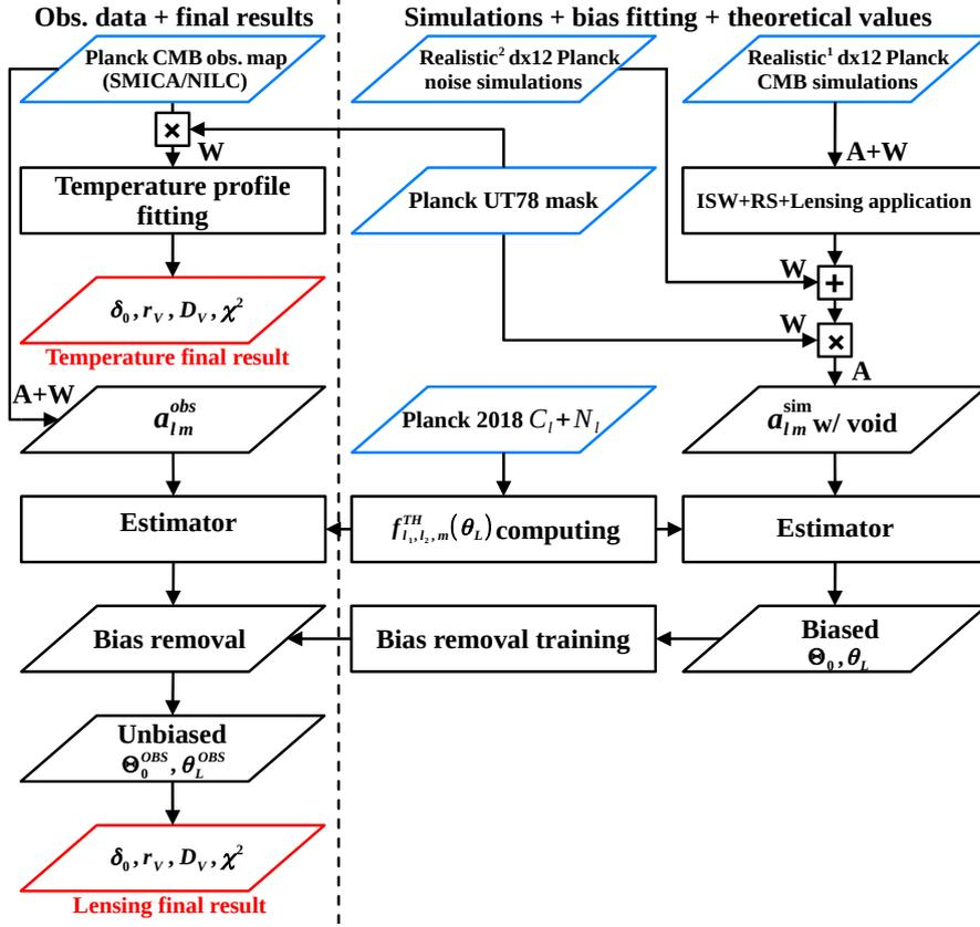
**Figure 7:** Our main pipeline. Blue boxes are input files from Planck, red are the final outputs. *Left column:* path from observational data to the final results for lensing and temperature. *Middle and right columns:* path from Planck simulations to the mock simulations with ISW, RS and lensing applied,  $f_{\ell_1, \ell_2, m}^{TH}$  computation and bias removal. W means a Wigner rotation (pointing the void to the north pole) and A the  $a_{\ell m}$  calculation with HEALPix’s Anafast.
