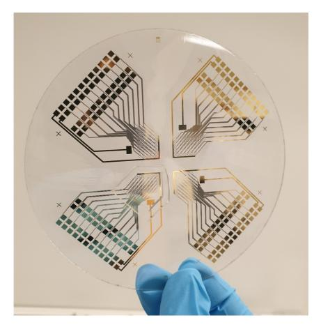
Figure S7. Glass wafer patterned with four EOECT classifiers.
