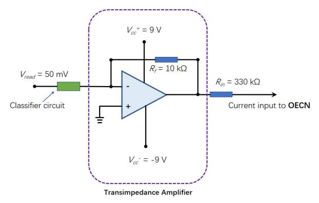
**Figure S6.** A transimpedance amplifier is used to interface the classifier and the OECN artificial neuron. Depending on the reading of the classifier, the amplifier delivers either a positive or negative current to the OECN.
