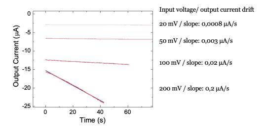
**Figure S8.** Evaluation of the drift upon the application of a positive read voltage in a solution of 1 mg/mL ETE-S with an applied gate voltage of 0 V.
