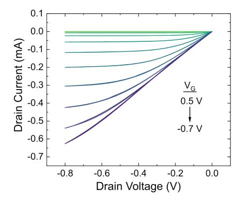
**Figure S10.** Output characterization of the device in Figure 2b, acquired in a solution of 100 mM NaCl.
