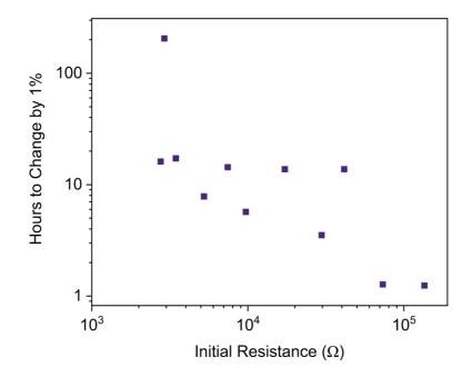
Figure S2. Time required for the current to change by 1%, as a function of the channel resistance. The highest point (206 hours) was taken as an outlier to obtain an average time of  $9.5 \pm 6.3$  hours.
