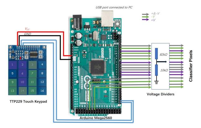
**Figure S3.** The touchpad setup for the "T/J" classifier training. The Arduino Mega 2560 microcontroller board is used to sample the touching signals from the keypad and deliver training pulses to the classifier through the voltage dividers.
