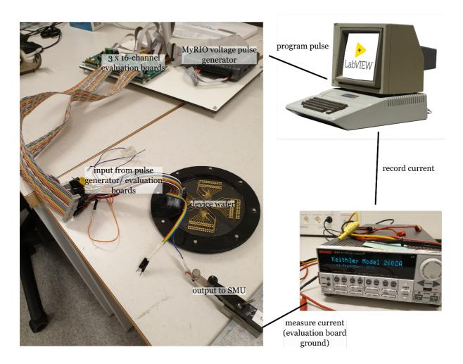
Figure S5. Classifier measurement setup.
