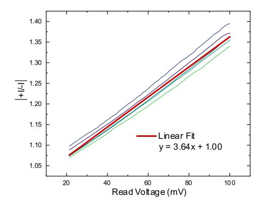
**Figure S1.** Current ratio between positive and negative voltages for a set of devices of varying conductance. Data taken from Figure 2e.
