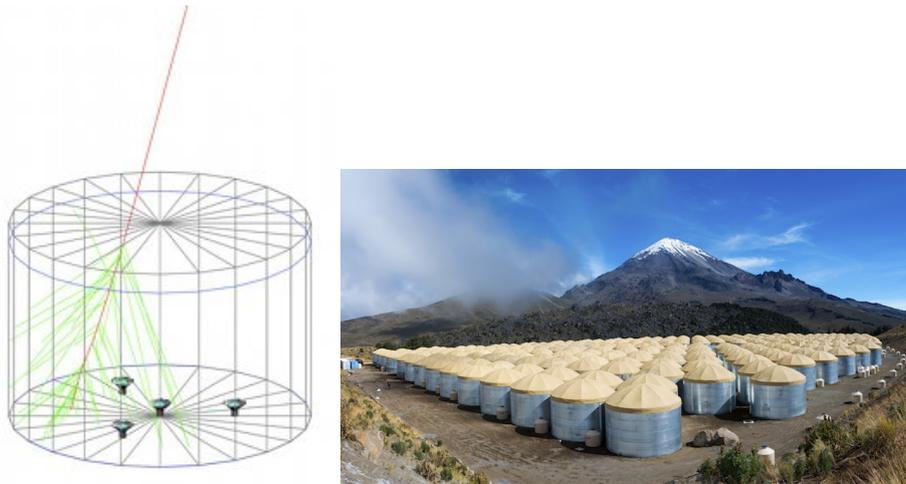
**Figure 24:** Water Cherenkov technique for EAS detection. Left: Simulation of a charged particle passing through a tank (red line) and emitting Cherenkov light (green lines). Also shown is the layout of the light sensors of the HAWC experiment, from the HAWC public website. Right: The HAWC Observatory (J. Goodman, Nov. 2016).
