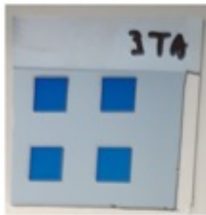
Fig.2 Prototype of charge selective contacts 2 x 2 device (each having 4 x 4 mm 2 area) array deposited on glass
