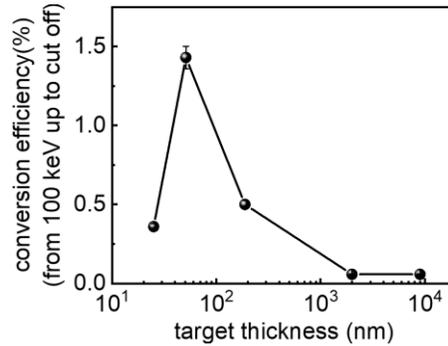
Fig. 7. Dependence of the conversion efficiency of laser energy into protons with energies above 100 keV on the thickness of *Al* targets in FWD direction at a 45° laser incidence angle (derived from Fig. 6).
