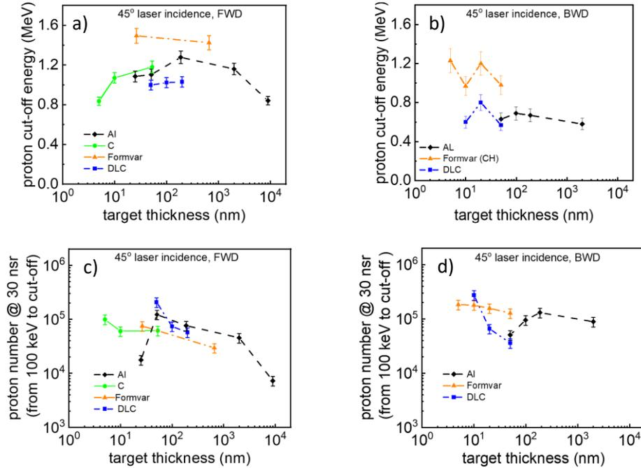
Fig. 3. (a), (b) the maximum energy of protons and (c), (d) highest number of protons versus thickness of the target emitted in forward (a), (c) ) and backward (b), (d)) directions are shown at  $45^\circ$  laser incidence angle on different target materials.
