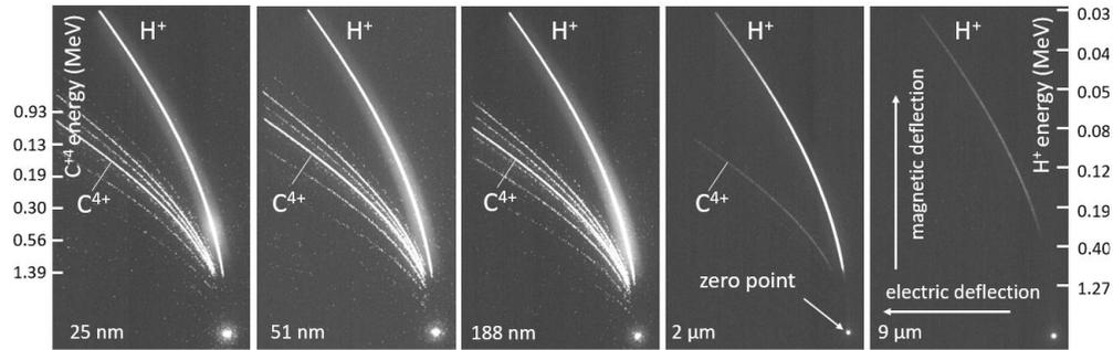
Fig. 5. The emitted ions spectral parabolic traces from *Al* target measured in the FWD direction at four successively increasing thicknesses with the highest proton cut off energy.
