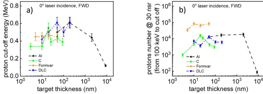
Fig. 4. a) The maximum energy of protons and b) the highest number of protons versus thickness emitted of the target in forward direction are shown at 0° laser incidence angle on the target for different target materials
