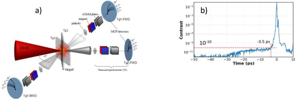
Fig. 1. a) The experimental arrangement. Laser incidence angle on target Tg1 and Tg2 is 45° and 0°, with respect to target normal direction, respectively. Thomson spectrometers are located in a rear or front surface target normal direction: from Tg1 the ions are measured in Tg1-FWD and in Tg1-BWD directions and from Tg2 in Tg2-FWD direction. b) The measured temporal contrast of the laser pulse.
