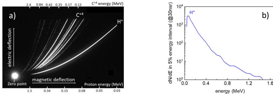
Fig. 2. (a) A typical CCD picture of measured ion spectra from a 26 nm formvar target, as an example, and (b) the evaluated proton spectrum (the background is subtracted).
