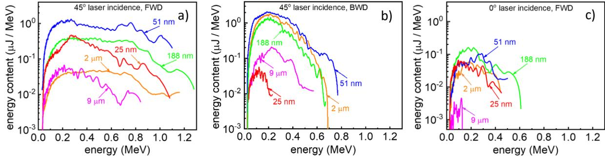
Fig. 6. The spectral energy content in the proton beam from *Al* targets at different thicknesses for FWB and BWD directions at 45° laser incidence and for FWD at 0° incidence.
