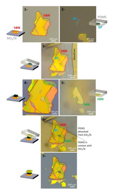
**Figure SM5a** - Optical images and associated diagrams describing the manufacturing process of a hBN/BP/hBN heterostructure: 1- Crystal of hBN on  $SiO_2/Si$ . 2- Crystal of BP on PDMS. 3- BP transfer on hBN, the wavefront corresponds to the PDMS -  $SiO_2/Si$  contact line. 4- BP/hBN heterostructure on  $SiO_2/Si$ . 5- hBN crystal on PDMS. 6- Transfer of hBN on BP/hBN. 7- hBN/BP/hBN heterostructure.
