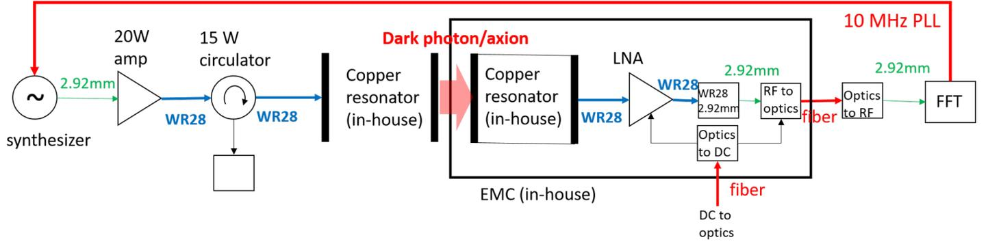
Figure 5: Schematic diagram of proof-of-principle experiment.
