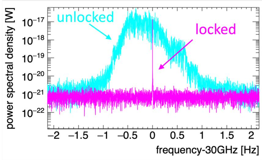
Figure 3: Demonstration of phase locking. The blue plot shows free running spectrum without the phase lock. The magenta plot shows virtually a  $\delta$ -function thanks to the phase-lock scheme investigated in this work.
