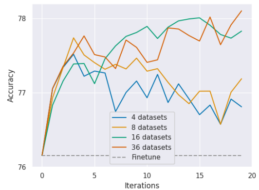
Figure 12: Number of datasets effect. The graph follows the performance (y-axis) per iteration (x-axis) during CoLD Fusion. Each color depicts a different number of datasets pool from where the datasets were randomly picked at each iteration. The pretrained model performance is highlighted by another dashed line.
