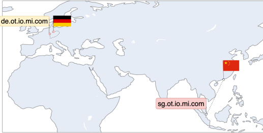
Fig. 6: Xiaomi Camera connects to two different domains when registered in China ( sg.ot.io.mi.com ), and in Germany ( de.ot.io.mi.com ). The domains were resolved to two different IP addresses in different geographical locations, correlated to the user-defined locations.
