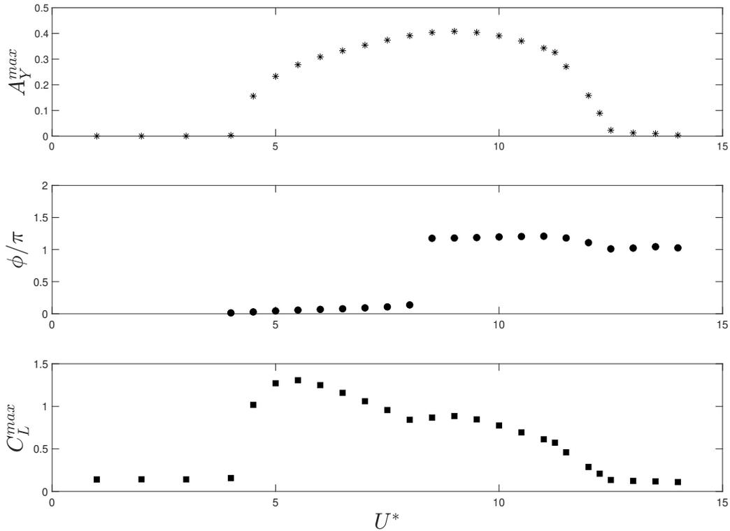
FIG. 20: Variation of maximum transverse displacements( $A_y^{max}/D$ ),  $\Phi$  and  $C_L^{max}$  at a gap ratio of  $g/D = 0.4$  with  $U^*$  for  $m^* = 10$  and  $Re = 100$
