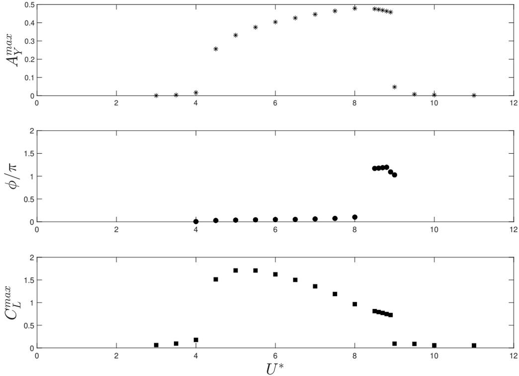
FIG. 18: Variation of maximum transverse displacements ( $A_y^{max}/D$ ),  $\Phi$  and  $C_L^{max}$  at a gap ratio of  $g/D = 0.5$  with  $U^*$  for  $m^* = 10$  and  $Re = 100$
