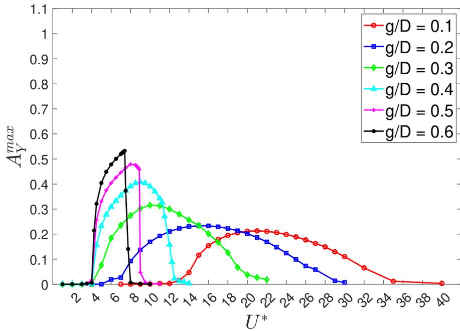
FIG. 4: Variation of maximum transverse displacements( $A_y^{max}/D$ ) with  $U^*$  for  $Re = 100$ ,  $m^* = 10$  and  $\zeta = 0$ .
