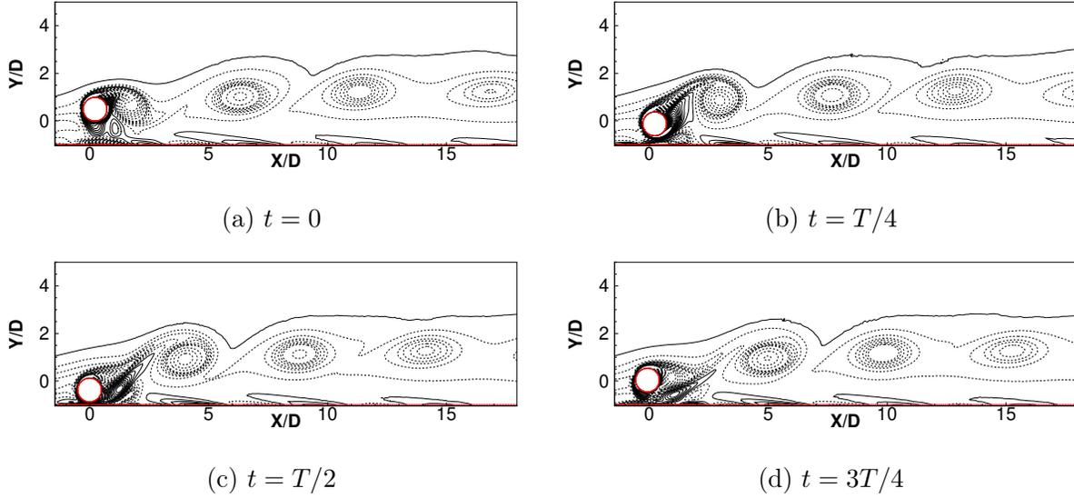
FIG. 7: Vortex shedding pattern at four equally spaced time snapshots a)  $t = 0$ , b)  $t = T/4$ , c)  $t = T/2$  and d)  $t = 3T/4$  for  $U^* = 7$  and  $g/D = 0.5$  at  $Re = 100$ , where  $T$  represents time period of one transverse oscillation of the cylinder
