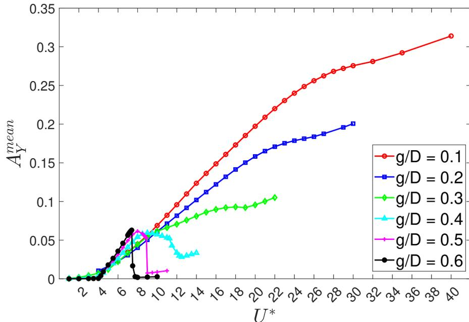
FIG. 6: Variation of dimensionless mean transverse displacement ( $A_Y^{mean}/D$ ) with  $U^*$  for  $Re = 100$ ,  $m^* = 10$  and  $\zeta = 0$ .
