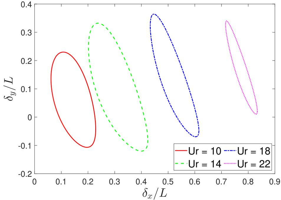
FIG. 16: The x-y trajectory of the cylinder at different  $U^*$  values at a gap ratio  $g/D = 0.2$
