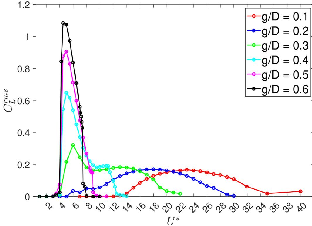
FIG. 12: Variation of root-mean-squared lift coefficient ( $C_L^{rms}$ ) with  $U^*$  for  $Re = 100$ ,  $m^* = 10$  and  $\zeta = 0$ .
