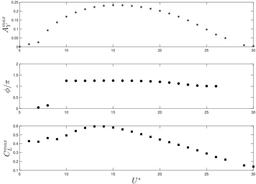
FIG. 22: Variation of maximum transverse displacements ( $A_y^{max}/D$ ),  $\Phi$  and  $C_L^{max}$  at a gap ratio of  $g/D = 0.2$  with  $U^*$  for  $m^* = 10$  and  $Re = 100$
