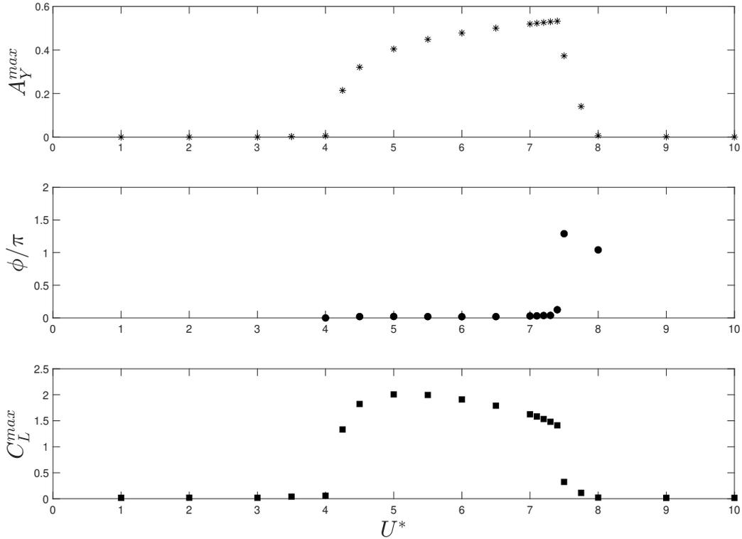
FIG. 17: Variation of maximum transverse displacements ( $A_y^{max}/D$ ),  $\Phi$  and  $C_L^{max}$  at a gap ratio of  $g/D = 0.6$  with  $U^*$  for  $m^* = 10$  and  $Re = 100$
