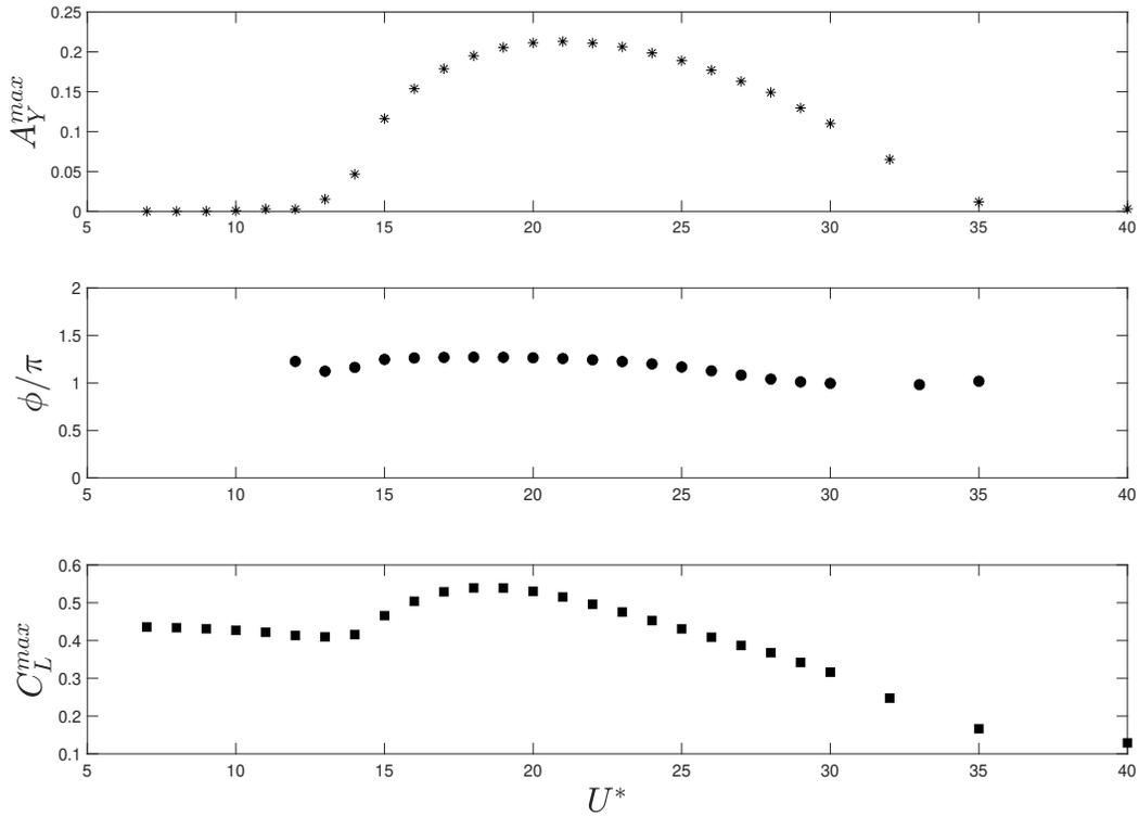
FIG. 24: Variation of maximum transverse displacements ( $A_y^{max}/D$ ), phase angle  $\Phi$  and maximum lift coefficient  $C_L^{max}$  at a gap ratio of  $g/D = 0.1$  with  $U^*$  for  $m^* = 10$  and  $Re = 100$
