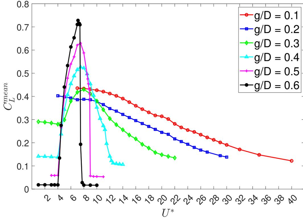
FIG. 10: Variation of mean lift coefficient ( $C_L^{mean}$ ) with  $U^*$  for  $Re = 100$ ,  $m^* = 10$  and  $\zeta = 0$ .
