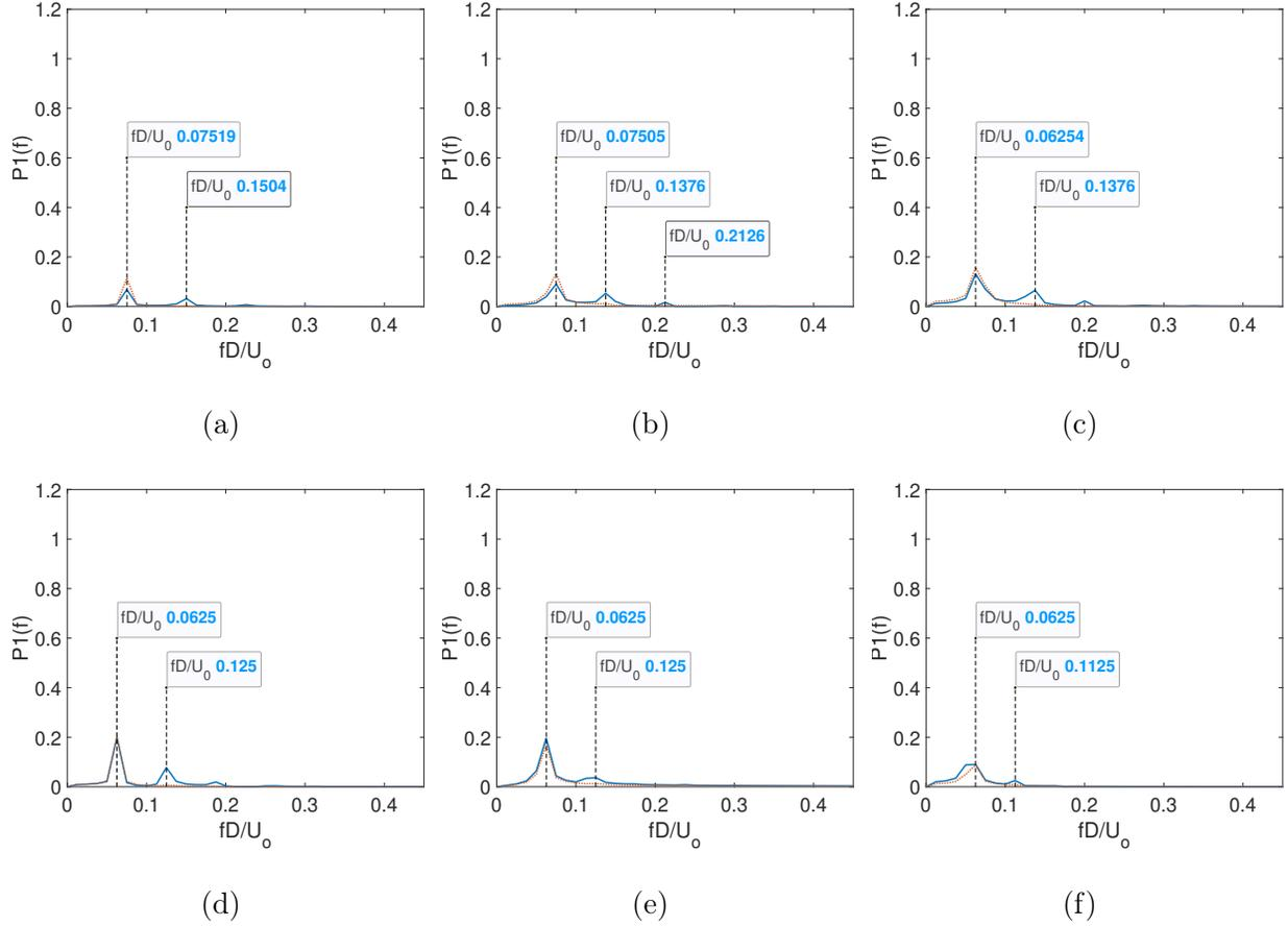
FIG. 25: Fast Fourier transform (FFT) of the lift force response for different  $U^*$  values at a gap ratio of  $g/D = 0.1$  for  $m^* = 10$  and  $Re = 100$ . a)  $U^* = 15$ , b)  $U^* = 16$ , c)  $U^* = 18$ , d)  $U^* = 20$ , e)  $U^* = 25$ , f)  $U^* = 30$ . (bold line represents lift force and dotted line represents displacement)
