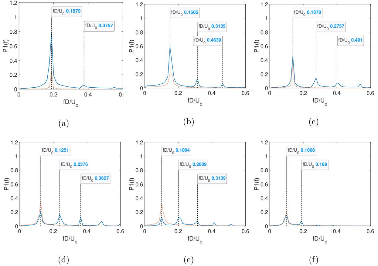
FIG. 23: Fast Fourier transform (FFT) of the lift force response for different  $U^*$  values at a gap ratio of  $g/D = 0.4$  for  $m^* = 10$  and  $Re = 100$ . a)  $U^* = 5$ , b)  $U^* = 6$ , c)  $U^* = 7$ , d)  $U^* = 8$ , e)  $U^* = 10$ , f)  $U^* = 11.5$ . (bold line represents lift force and dotted line represents displacement)
