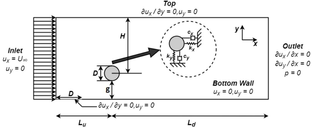
FIG. 1: Schematic of computational domain and boundary conditions for freely vibrating cylinder near stationary wall
