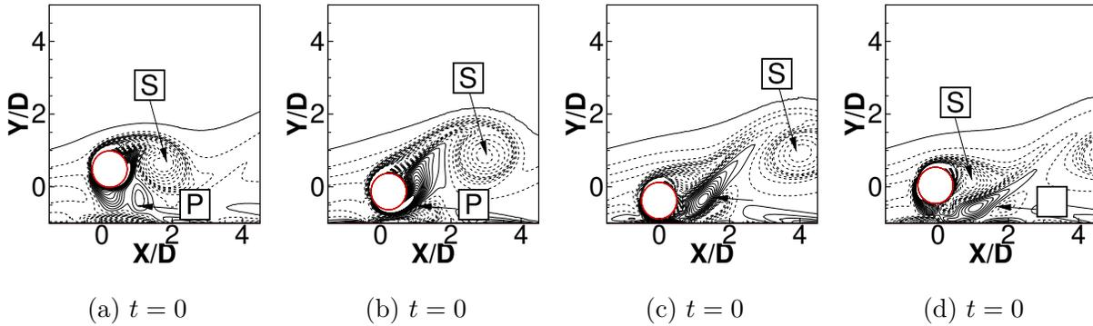
FIG. 8: Vortex shedding pattern at four equally spaced time snapshots a)  $t = 0$ , b)  $t = T/4$ , c)  $t = T/2$  and d)  $t = 3T/4$  for  $U^* = 7$  and  $g/D = 0.5$  at  $Re = 100$ , where  $T$  represents time period of one transverse oscillation of the cylinder
