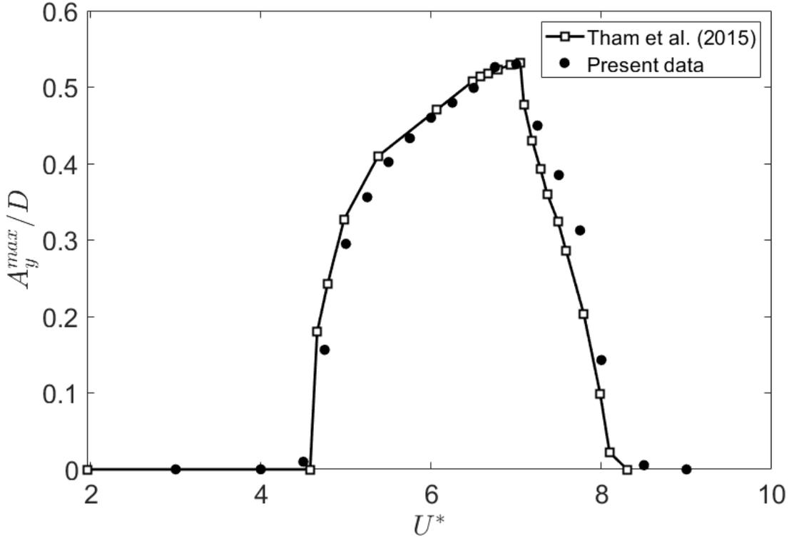
FIG. 2: Comparison of maximum transverse amplitude with [30] for a cylinder near the wall at  $m^* = 10$ ,  $\zeta = 0$ ,  $g/D = 0.75$  &  $Re = 100$ .
