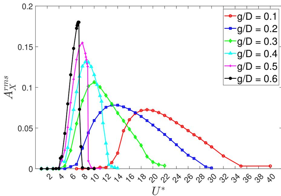
FIG. 5: Variation of root-mean-squared stream-wise displacement( $A_X^{rms}/D$ ) with  $U^*$  for  $Re = 100$ ,  $m^* = 10$  and  $\zeta = 0$ .
