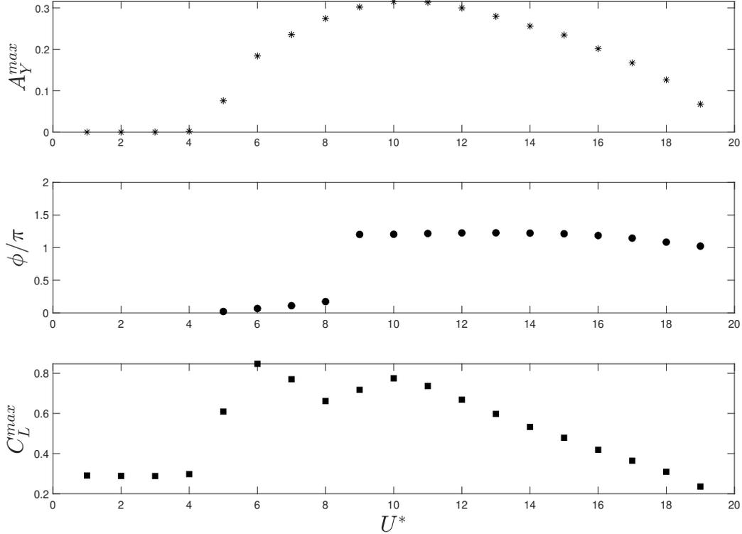
FIG. 21: Variation of maximum transverse displacements ( $A_y^{max}/D$ ),  $\Phi$  and  $C_L^{max}$  at a gap ratio of  $g/D = 0.3$  with  $U^*$  for  $m^* = 10$  and  $Re = 100$
