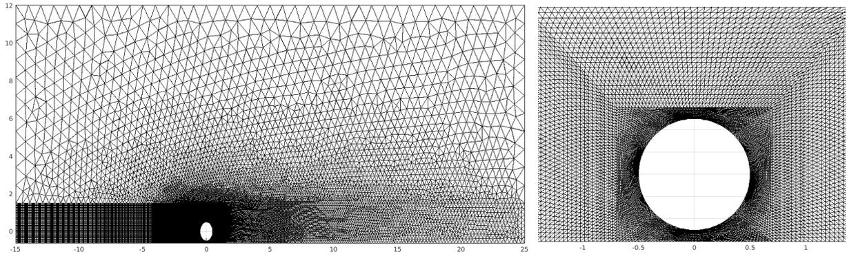
FIG. 3: The typical quadratic six-noded triangular fluid mesh considered for the gap-ratio of  $g/D = 0.1$  (left) and closeup view of the mesh around the circular cylinder (right).
