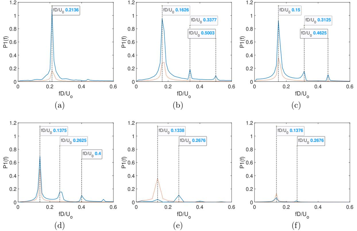
FIG. 19: Fast Fourier transform (FFT) of the lift force response for different  $U^*$  values at a gap ratio of  $g/D = 0.6$  for  $m^* = 10$  and  $Re = 100$ . a)  $U^* = 4.25$ , b)  $U^* = 5.5$ , c)  $U^* = 6$ , d)  $U^* = 7$ , e)  $U^* = 7.5$ , f)  $U^* = 7.75$ . (bold line represents lift force and dotted line represents displacement)
