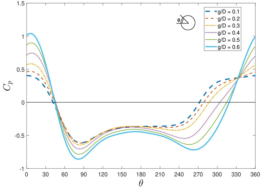
FIG. 11: Variation of  $C_p$  along the surface of the circular cylinder in the pre lock-in region for  $Re = 100$ ,  $m^* = 10$  and  $\zeta = 0$ . Here  $\theta = 0$  starts from the negative x axis and varies in the clockwise direction.
