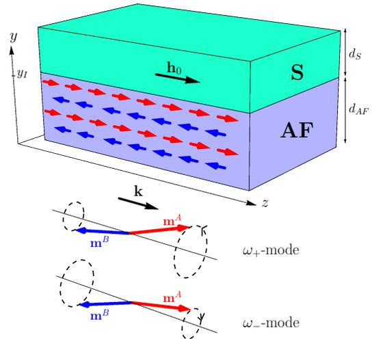
FIG. 1. Sketch of the AF/S bilayer under consideration and a schematic illustration of the circularly-polarized magnon modes, which are energetically degenerate without a coupling to the S(N) layer and an applied magnetic field.
