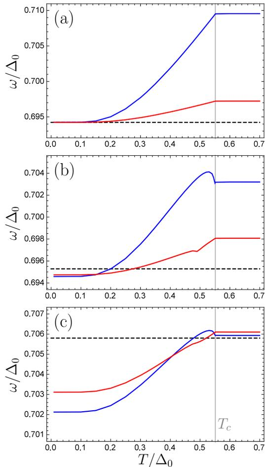
FIG. 3. Dependence of the mode frequencies  $\omega_+$  (blue) and  $\omega_-$  (red) on temperature for three representative values of the magnon wave number  $k$ : (a)  $k = 0$ , (b)  $kc/2 = 0.009$ , (c)  $kc/2 = 0.03$ . For all panels black dashed line is  $\omega_0$ . Vertical grey line marks the superconducting critical temperature of the AF/S bilayer.  $h_0 = 0.2\Delta_0$ .
