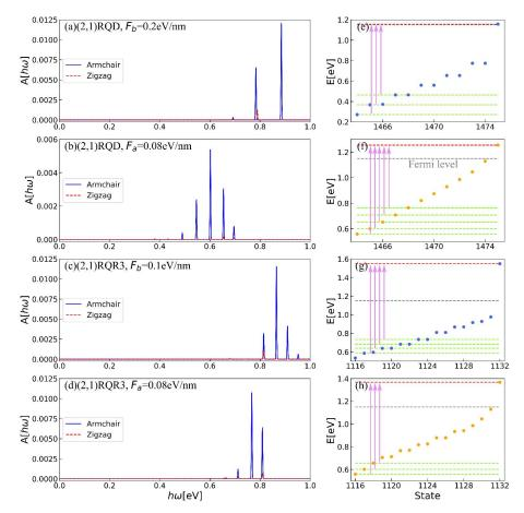
**Fig.12.** Optical absorption spectra of (2,1)RQD[(a)(b)], (2,1)RQR3[(c)(d)]. In (e)(f)(g)(h), the grey dashed line indicates the Fermi level, which is tuned to 1.15eV between the lowest bulk state and the highest  $\delta$ -P dominated edge
