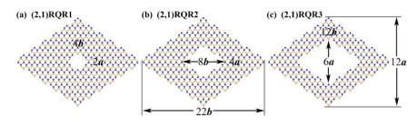
Fig.3. A collection of (2,1) RQRs with different widths (the distance between the inner and outer edge).
