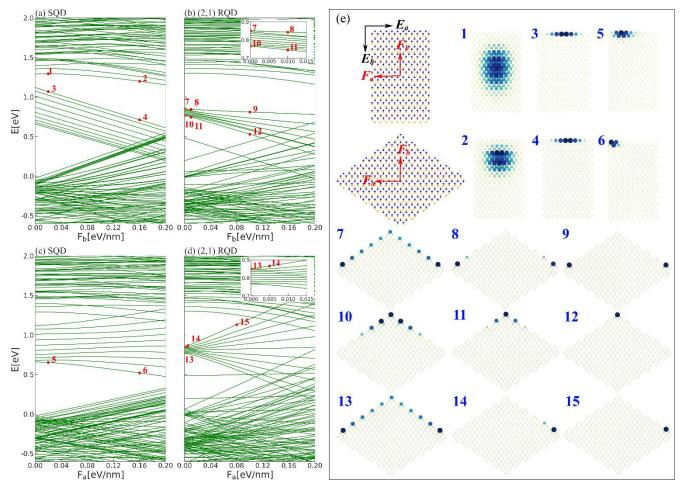
**Fig.6.** The energy spectra of SQD and (1,2)RQD as a function of in-plane *b*-direction and *a*-direction increasing electric field, respectively.
