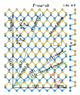
**Fig.1.** Schematic illustration of monolayer b-AsP QD. The red rectangle refers to the unit cell of b-AsP; **a** and **b** are the lattice constants; the chiral vector **T** is illustrated by the thick solid arrow along each 2D crystallographic direction; *R*<sub>1</sub>-*R*<sub>7</sub> are the seven hopping parameters.
