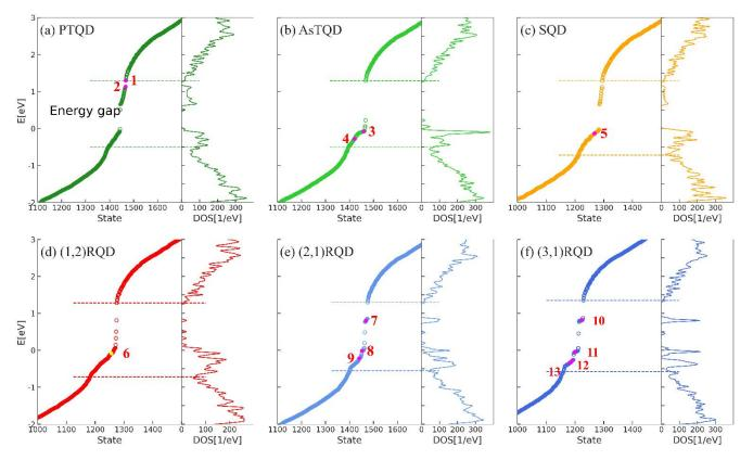
**Fig.4.** The energy levels of P/AsTQD, SQD, (1,2)/(2,1)/(3,1)RQD around the energy gap. The corresponding probability densities of the marked states are shown in Fig.5.
