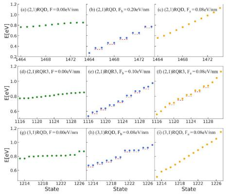
**Fig.7.** The energy levels of (2,1)RQD, (2,1)RQR3, and (3,1)RQD without external field and with transverse electric field along **a** and **b** directions.
