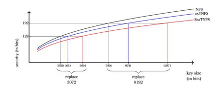
Fig. 2 Modification of key sizes according to the O(1)-less formula [26]
