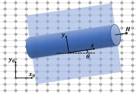
FIG. 1. A schematic of a chiral nanotube formed by rolling a two-dimensional sheet. The two coordinate systems,  $(x_0, y_0)$  and  $(x, y)$ , are connected by a rotation of the chiral angle  $\theta$ . A magnetic field  $\mathbf{H}$  is applied along the tube to generate nonreciprocal effects.
