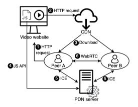
Figure 1: Traffic flows of a typical PDN scenario.
