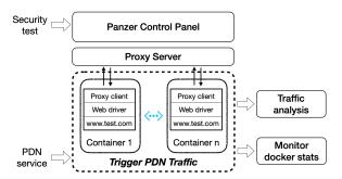
Figure 2: The architecture of the PDN Analyzer
