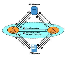
Figure 4: Illustration of IP exchange in PDN
