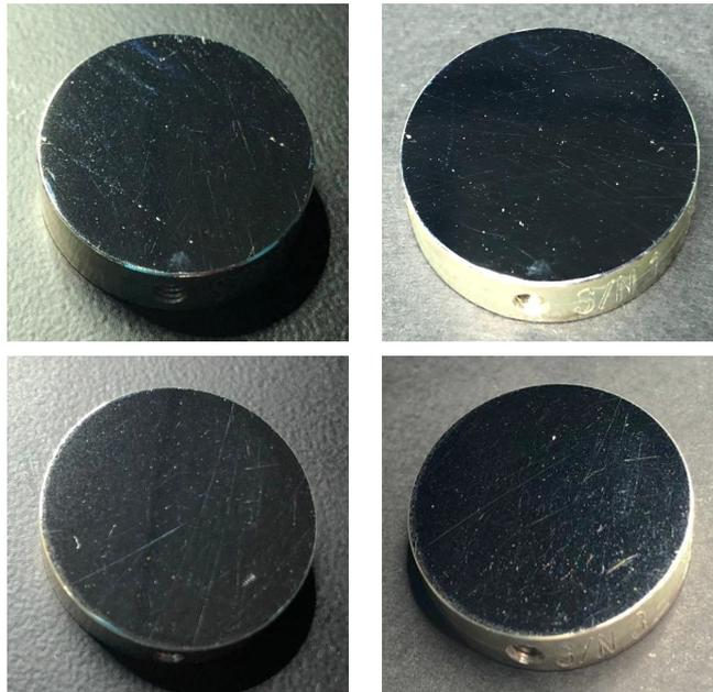
**Figure 3.2:** Pictures of the samples taken before (left) and after (right) the cryogenic cycles. The spot marked with a red oval is a reflection artifact from the lamp used for the inspection, and not a surface blemish.
