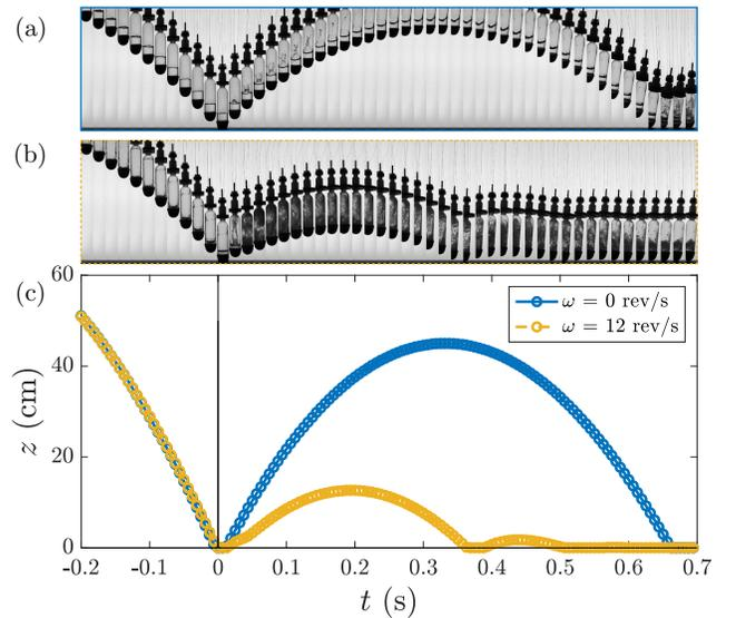
Figure 1. Impact of partially filled containers. (a) Sequence of images for a container dropped with a quiescent fluid inside. (b) Sequence when the container is rotated at frequency  $\omega = 12$  rev/s before release. (c) Trajectories for the lowest point of the container, for the same time interval as panels (a) and (b).
