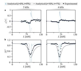
Figure 5. Comparison between the experimental and analytical (a) phase modulation results and (b) transmission ratios.
