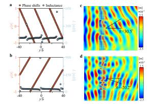
Figure 6. Metasurface with single-resonant shunts for deflecting normally incident  $A_0$  mode Lamb wave. The phase profile and the required inductance values along metasurface for (a) 5 kHz and (b) 6 kHz wavefront deflection.  $\bar{b} = 7$  mm represents the distance between adjacent units. The out-of-plane displacement wavefields of the wave-deflecting metasurface ((c): 5 kHz, (d): 6 kHz).
