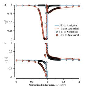
Figure 3. Transmission characteristics of the metasurface unit with multi-resonant shunts. (a) Transmission ratios changing with normalized inductance,  $L_1/(\omega_m^2 C_p^{eq})$ . (b) Phase modulation curves of 5 kHz and 10 kHz flexural waves showing a similar trend.
