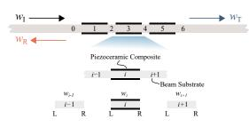
Figure A1. Schematic of the metasurface unit and piezoelectric bimorphs with superscripts R and L denoting right and left boundaries.
