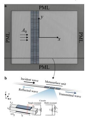
Figure 1. Schematic of (a) piezoelectric-based electroelastic metasurface embedded in a plate and (b) the metasurface unit. The perfectly matched layers (PMLs) are implemented to simulate the infinite domains. The inset in (b) shows the piezoelectric bimorph with resonant shunt circuits.
