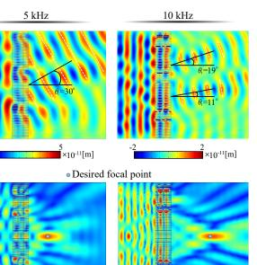
Figure 8. Metasurface with multi-resonant shunts. (a) The out-of-plane displacement wavefields of the multi-resonant deflecting metasurface under different frequency incident waves demonstrating a smaller angle under higher frequency excitation. (b) |w| wavefields of the multi-resonant focusing metasurface under different frequency incident waves, validating that the wave intensity is localized at the desired region.
