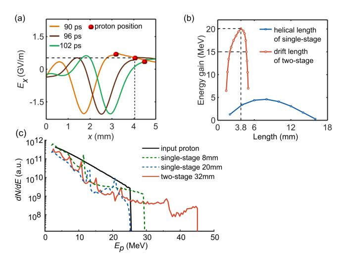
Figure 8. (a) snapshots of the current distribution and the positions of protons in HC, at 90 ps, 96 ps and 102 ps. (b) Energy gain by varying the helical length of single-stage and the drift length of two-stage HC. (c)Spectrum of the input protons (black line); spectrum after a single-stage HC of 8 mm (green dashed line) and 20 mm (blue dashed line); spectrum after a two-stage HC (red line).
