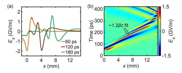
Figure 3. (a) Snapshot of the longitudinal electric field on the central axis of HC at 60 ps, 120 ps, and 180 ps.(b) Spatial-temporal distribution of the longitudinal electric field in an HC, with the mark of extreme points of positive fields (green dashed lines).
