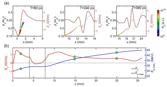
Figure 7. (a) Snapshots of the protons' phase space  $(x, p_x)$  and  $E_x$  at 60 ps, 240 ps and 360 ps, in the two-stage HC. (b) Longitudinal electric field in the coordinate frame of the traveling highest-energy protons (red curve) and the evolution of the maximum energy (blue curve) in two-stage HC, the three groups of green circles mark the three snapshots in (a).
