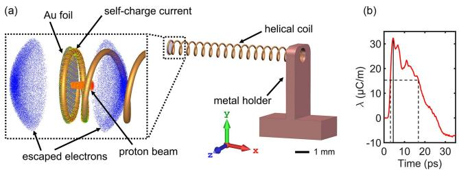
Figure 1. Simulation setup of (a) HC target configurations and (b) the self-discharged current generated by the emitted particles.
