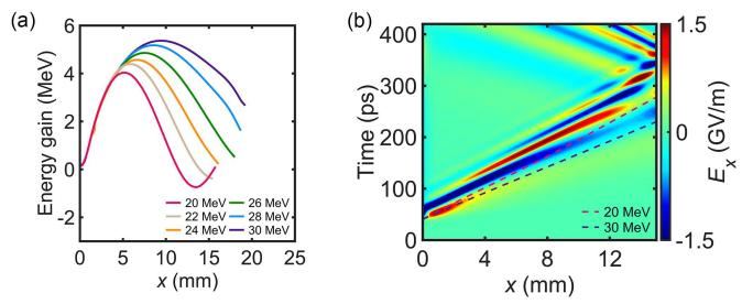
Figure 5. (a) Energy gains of traveling protons in HC with input energies. (b) The spatial-temporal distribution of  $E_x$  and trajectories of protons with different input energies.
