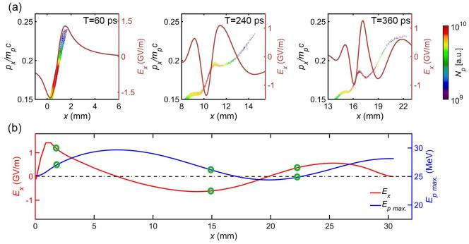
Figure 4. (a) Snapshots of the protons' distribution in phase space  $(x, p_x)$  and the longitudinal electric field at time of 60 ps, 240 ps and 360 ps, in single-stage HC. (b) Longitudinal electric field in the coordinate frame of the traveling highest-energy protons (red curve) and the evolution of the maximum energy (blue curve) in single-stage HC, the three groups of green circles mark the three statuses in (a).
