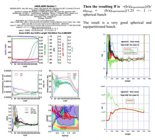
Fig. 28.4. Sine vanes. ffadj = 0.80\*(4th order polynomial fit)  $\sim (b/a)_{experimental})/(b/a)_{design} = (b/a)_{experimental})/1.25 = \sim 1 -> spherical bunch.$
