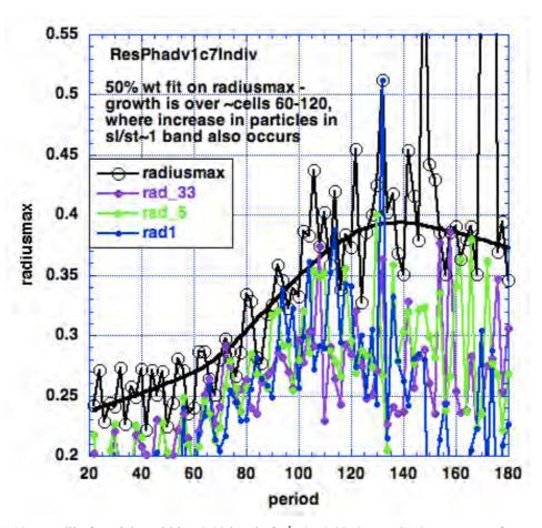
Fig. 21.10.a. Radii of particles within  $\pm 0.03$  band of  $\sigma^l/\sigma^t = 0.33$ , 0.5, and 1.0 resonances for particles being transmitted at each period. Radiusmax is the maximum radius of all particles at that period, solid line is 50% weighted fit. A particle in band near  $\sigma^l/\sigma^t = 0.33$  is at maximum radius at period 66, 72, 108 and 158; near  $\sigma^l/\sigma^t = 0.5$  at cell 166, and near  $\sigma^l/\sigma^t = 1.0$  at cell 132.
