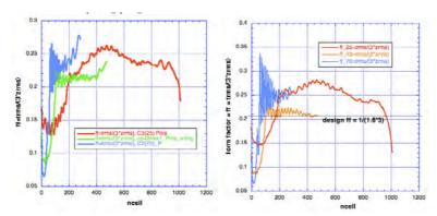
Fig. 22.22. Space charge form factor (trms/(3\*zmrs). a. full Poisson b. "2-term"
