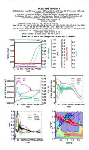
Fig. 28.7. 2term Vanes. ffadj to make spherical bunch. Length 708 cm.
