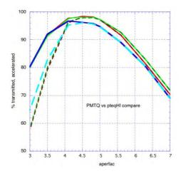
Fig. 15.1 Aperfac comparison of PARMTEQM and pteqHI with same basic procedures except for the independent variable and residual paraxial approximation in PARMTEQM. Red-PARMTEQM with individual particle paraxial approximation in dynamics. Green PARMTEQM with no paraxial approximation. Blue and light blue - pteqHI. Solid lines are transmission, dashed are accelerated fraction.
