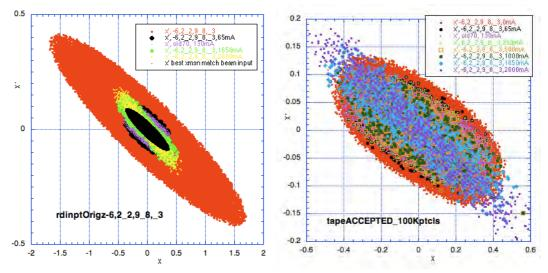
Fig. 19.34 Dynamic aperture vs. beam current.
