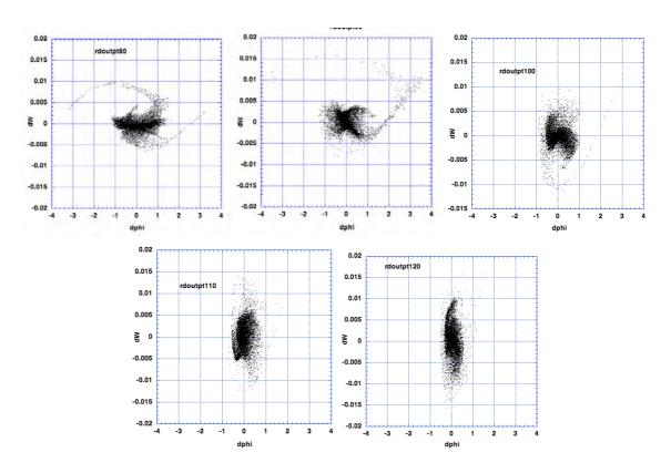
Fig. 21.8. dphi-dW phase space of individual particles at end of cells 80, 90, 100, 110, 120.
