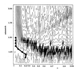
Fig. 24.17.b. Contour plot of maximum halo radius, per Fig. 24.17.a. Dots connected by lines are threshold points determined by the resonance width method.
