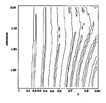
Fig. 24.18. Central density oscillation wavelength scaled to (betatron wavelength)/sqrt(4 - 2µ).
