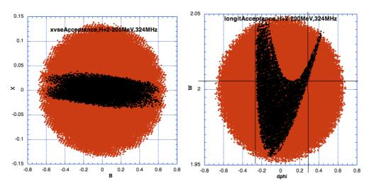
Fig. 11.1.3. a. Transverse acceptance of a 2-200MeV, 324 MHz H+ APF linac. b. Longitudinal acceptance.
