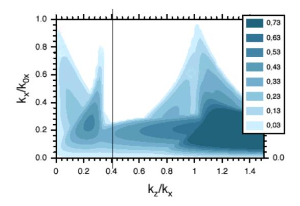
Fig. 5.2.3-1. Hofmann Chart for longitudinal-to-transverse emittance ratio eln/etn = 2.0; thus kz/kx = 0.5 is the equipartitioned condition for this chart.
