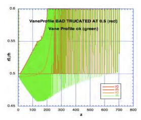
Fig. 29.2 The 2-term vane profiles. Green - Standard design. The minimum radius = 0.46 cm at the end of the standard shaper, then increases. Red – vane radii below 0.5 cm cut off (truncated).
