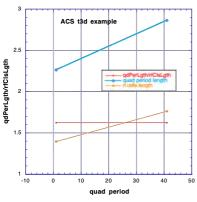
Fig. 27.24. Total length of quad periods and lengths occupied by rf sections and quad with associated drifts. Average transverse focusing period length ~ 2.5 meters. 3 meters is used in graphs below for representative values of (phase advance/(transverse focusing period length)
