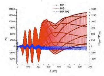
Fig. 17.43 Longitudinal kicks from multipole expansion method and multigrid Poisson solver on a certain particle along the RFQ.
