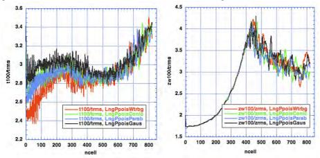
Fig. 22.7. For Long Focusing Channel With Bunching Followed by Accelerating Channel: The ratios of a.) 100% transverse beam size to the transverse beam size (t100/trms) and b.) corresponding longitudinal ratio (zw100/zrms).
