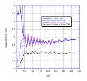
Fig. 6.2-4. Equipartitioning ratio, and corresponding beam size, emittance and tune ratios, Eqs. (7) and (8) for the Post-CDR equipartitioned RFQ using pteqHI including multipole and image-charge effects.
