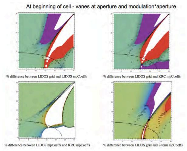
Fig. 16.4 Contour plots of the potential difference between Poisson and multipole solutions.
