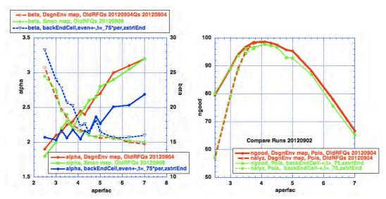
Fig. 19.48 Comparison of best input transmission match, design envelope match, and backward simulation input match. Left – input match ellipse alphas and betas. Right - full Poisson simulation with trnsmission matches for RFQ family, with a 2-cell input section consisting of an entrance wall with hole and then a large aperture section, before the start of the vanes. ngood = transmitted particles, nalyz = accelerated articles, from a 10,000 particle input distribution.
