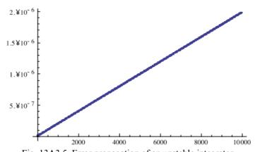
Fig. 13A3.5 Error propagation of an unstable integrator.
