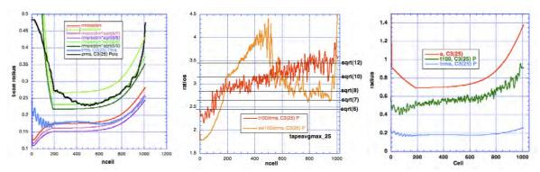
Fig. 22.21. Case 3(25) full Poisson simulation. a. rms beam sizes, design waterbag beam sizes and adjusted design beam sizes. b. 100% to rms beam size ratios. c. t100 and trms size beam sizes compared to aperture.
