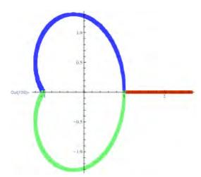
Fig. 13A3.4 Root locus diagram of an unstable integrator.
