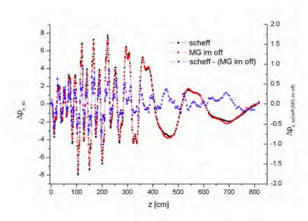
Fig. 17.47 Transverse space charge kicks from scheff and the multigrid Poisson solver.
