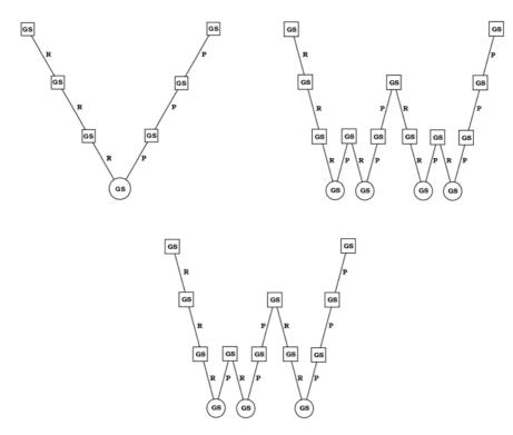
Fig. 17.3 a. V-cycle, b. W-cycle, c. F-cycle.
