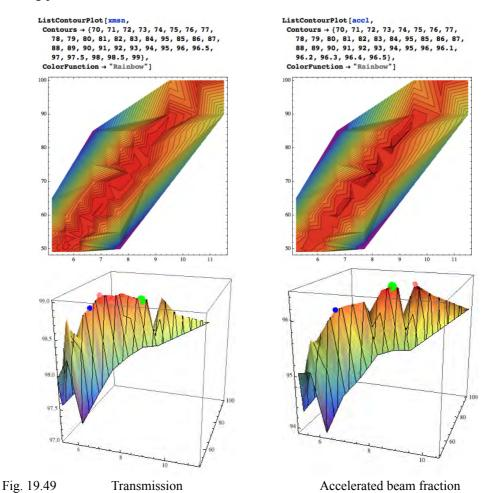
Advanced input matching strategies are a unique feature of *LINACS*. As a demonstration background, arrays of transmission (xmsn) and accelerated beam fraction (accl) vs. {alpha,beta} were made, requiring many full Poisson runs (very tedious). Because of the long entrance wall, the area of good matches is an unusual long, narrow peak. Fig. 19.49 The highest transmission point of this rather coarse matrix search is {alpha 6.7, beta 60., xmsn 99.02, accl 96.23}, shown by the pink dot in Fig. 2.
