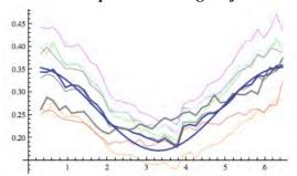
Fig. 19.40 Typical variations in the x-beam-size as the input ellipse a and b are varied. The smooth curve is the desired variation according to the RFQ design.
