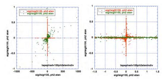
Fig. 21.5. Hofmann Chart for single particle 2-cell transverse phase advances in 6D phase space. Right is expanded horizontal scale.
