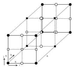
Fig. 17.4 Trilinear interpolation in 3D.
