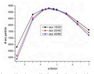
Figure 17.22: Space charge grid, no images: Number of accelerated particles as a function of the grid resolution (dr=aperture/x and dz=cell length/y). The external field grid uses the default settings of dr=aperture/20 and dz=celllength/40.
