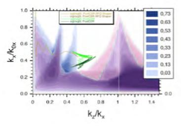
Fig. 6.2-5. Composite Hofmann Chart for eln/etn=1.4 (underlying blue-toned shadows) and eln/etn = 2 (overlying magenta toned shadows). The Post-CDR equipartitioned RFQ trajectories for the shaper and from the EOS to the output are shown, using pteqHI including multipole and image-charge effects.
