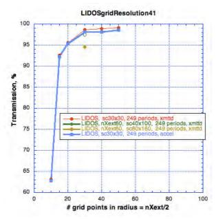
Fig. 18.2. Effect of the number of mesh points in the radius (nXext)/2 on transmission.
