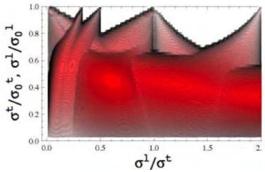
Fig. 1.2. Stability chart showing stop-bands for resonances at  $\sigma^l/\sigma^t$  near 0 and at 0.33, 0.5, 1.0 and 2.0. (Chart is for rms emittance ratio eln/etn=10.) (( $\epsilon_{ln}$ ,  $\epsilon_{tn}$ ,  $\sigma^t$ ,  $\sigma^l$  and the zero-current phase advances  $\sigma_0^t$  and  $\sigma_0^l$  may be simplified for typing by etn, eln, st, sl, s0t and s0l).
