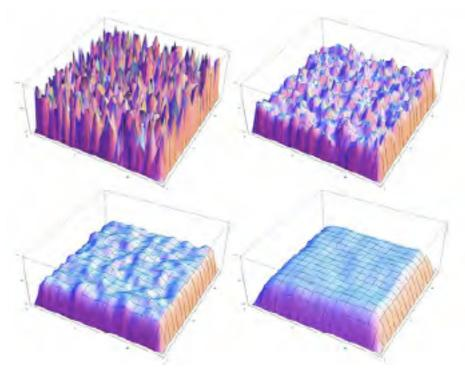
Fig. 17.1: Initial values and approximation after 1, 3, and 10 cycles. The high frequency components are sufficiently reduced, whereas the low frequency components remain.
