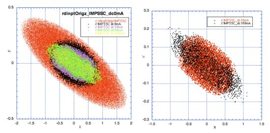
Fig. 19.32a. Red – the input dc distribution. Other distributions are the accepted particles for 0, 10, 50 and 100mA input particle currents.
