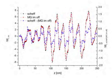
Fig. 17.48 Transverse space charge kicks from scheff and multigrid Poisson solver for the first 2:5 m.
