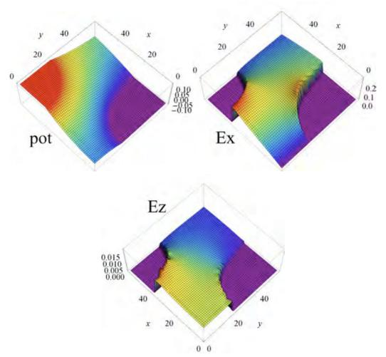
Fig. 17.28 XY-plane of the potential, Ex and Ez at the center of cell 400.
