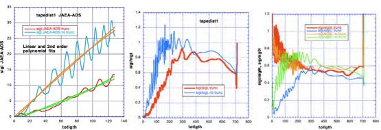
Fig. 29.20 Rms beam sizes, longitudinal total beam size, longitudinal phase advance sigl, tune ratios, and tune depressions. There is slightly more space charge effect with the truncated vanes.
