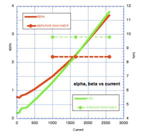
Fig. 19.35 Variation of dynamically accepted ellipse alpha and beta with input beam current.
