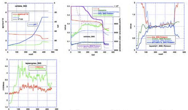
Looks like resonance ~cell100-150. Not EP at cell100, but EP at cell150. Probably continual longit loss up to ~cell 400. Scraping from ~cell200-380, especially at cell 380. On purpose?- flat parameters V and m, slight opening of aper. Old CURLI LBL design. No trms redistribution.
