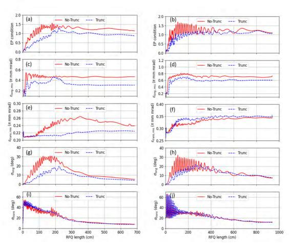
Fig. 29.16 Design comparison between truncated (Trunc) vane and No-truncated (No-Trunc) vanes for the JAEA-ADS EP RFQ (left) and the IFMIF CDR EP RFQ (right). (a) and (b) plot show the EP condition, (c) and (d) are the longitudinal normalized rms emittance, (e) and (f) are the transverse normalized rms emittance, (g) and (h) are the longitudinal phase advance, and (i) and (j) are the transverse phase advance.
