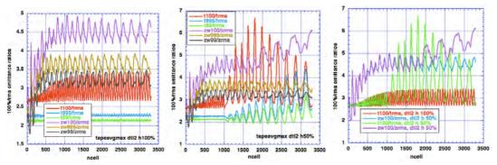
Fig. 27.10. Total/rms beam size ratios – 100% quads (left), – 50% quads (middle), – compare 100%/rms ratios (right). t100/trms with 50% quads becomes very large, and eventually the longitudinal zw100/zrms also increases.
