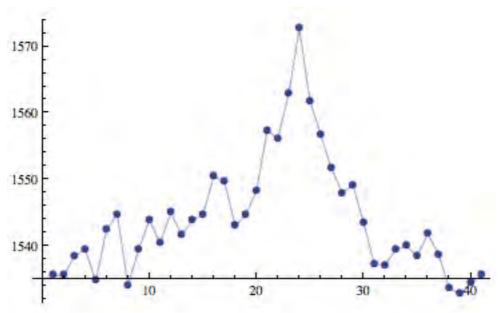
Fig. 19.14 Potential on the axis for standard beam with 10,000 particles. The difference between the maximum and minimum is 2.53%. The Poisson cycle variables are the standard m=5, n1 = n2 = 7. Using m=10, n1 = n2 = 14 doubled the running time (for a 10 cell run) but made no discernable difference in the potential on axis.
