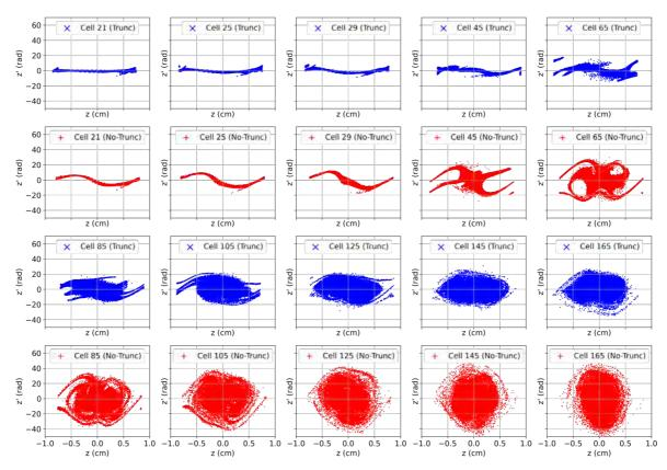
Fig. 29.23 Longitudinal phase distribution at different locations along the shaper section for Truncated vane (blue x) and No-truncated (red plus).
