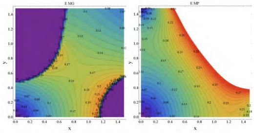
Fig. 17.38 Absolute value of the electric field (E) in the xy-plane at the end of a accelerating cell for multigrid Poisson solver and multipole expansion method.
