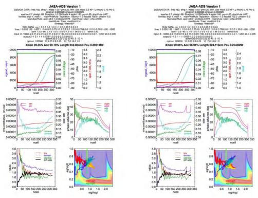
Fig. 23.7. The *LINACS* run graphic shows the important beam performance aspects. 10000 particles simulated. Left – 2term vane modulation, Right - Sine vane modulation. Dark blue line in upper left graph illustrates the transmission and accelerated beam. The longitudinal emittance growth, and corresponding transverse emittance growth are seen in each middle left graph, and tune depressions at lower right.
