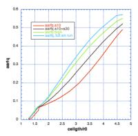
Fig. 23.10. Comparison of various acceleration term coefficients vs. (cell length)/r0 ratio through the RFQ, for a "typical" 0.035-2.5 MeV RFQ
