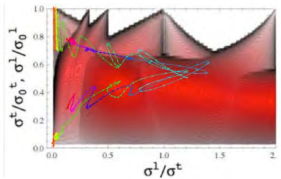
Fig. 1.4. Rms trajectories on Hofmann chart drawn for EP ratios eln/etn = b/a = sigt/sigl = 10. The trajectories progress from red at the RFQ input through orange, yellow, green, blue, magenta at the RFQ output. The chart shows stop-bands for resonances at  $\sigma^l/\sigma^t$  near 0 and at 0.33, 0.5, 1.0 and 2.0. Note that the influence of the sigl/sigt=1 resonance is very broad and strong, with tails extending far away from 1:1.
