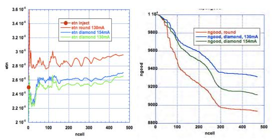
Fig. 22.6. Normalized transverse rms emittance and transmission for round or diamond-shaped input beams injected into an RFQ.
