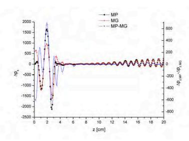
Fig. 17.44 Longitudinal kicks from multipole expansion method and multigrid Poisson solver on a certain particle along the beginning of the RFQ.
