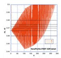
Fig. 29.14 IFMIF CDR RFQ sinusoidal modulation vane profile. The shaper ends at cell 116, z=103. The vane voltage is kept at the Kilpatrick level; the aperture increases rapidly after the shaper. Six truncations were tested; best truncation = 0.47, just above begin-shaper aperture.
