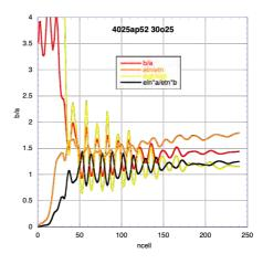
Fig. 19.3 The EP characteristics of an anecdotal 400 MHz preliminary design search. (The ripple like this is usually improved by better input transverse matching.)
