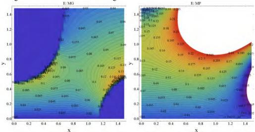
Fig. 17.36 X-component of the electric field (Ex) in the xy-plane at the end of a accelerating cell.
