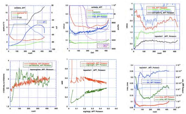
Parameters do not saturate, strange variations. Significant longitudinal losses, -> Case 3(25). No trms redistribution. 2term result clearly shows smaller trms and redistribution.
