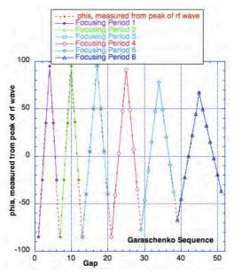
Fig. 7.1 Garaschenko APF sequence. Phis is measured from the peak of the wave.
