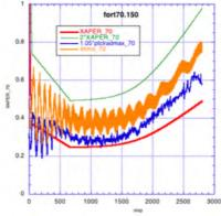
Fig. 14.7 Left – aperfac45 case, right – aperfac70 case. Four boundaries are shown: Red – XAPER, the minimum vane aperture. Green – 2\*XAPER (also the maximum aperture when the modulation = 2). Blue – 1.05\*(maximum particle radius (of particles successfully transmitted to the end of the RFQ). Yellow – Four times the transverse rms radius of particles successfully transmitted to the end of the RFQ.
