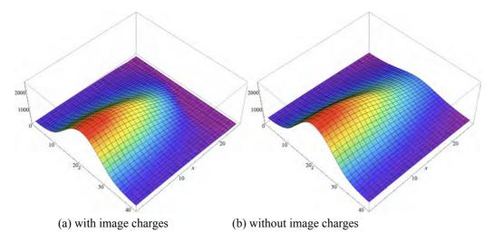
Fig. 17.51 Space charge potential at a xz-plane with and without image charges.
