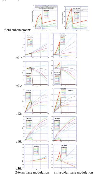
Fig. 23.16. Plots for field enhancement factor and multipoles from original K.R. Crandall tables for 2-term (standard) vs. sinusoidal vane tip modulation, to give a visual feeling for some of the differences.
