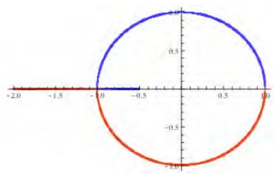
Fig. 13A3.1 Root-locus diagram for stable leapfrog integrator.
