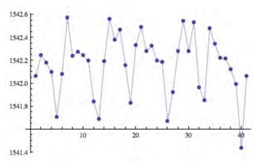
Fig. 19.16 Potential on the axis for standard beam with 1,000,000 particles. The difference between the maximum and minimum is 0.074%.
