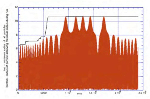
Fig. 24. 9. Mismatched Hamiltonian initial distribution, with mu = 0.54 and mismatch = 1.30. Maximum radius of all particles during the run, and radius of the particle that achieved the maximum radius during the run.
