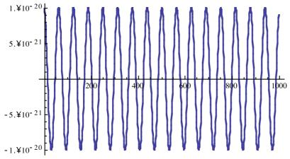
Fig. 13A3.2 Error propagation for stable leapfrog integrator.
