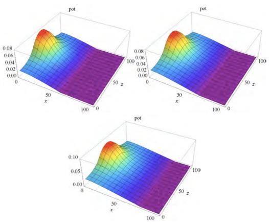
Fig. 17.17 Potential after 10 multigrid iterations of a 0.2 cm radius charged ball placed inside a quadrupole channel with aperture from 0.2 cm to 0.8 cm, increments 0.1 cm.
