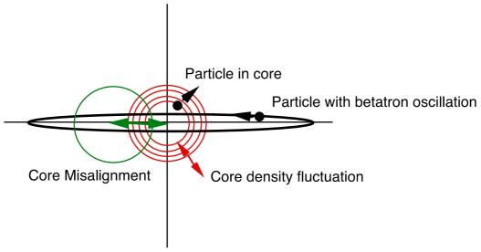
Fig. 24.1. Schematic of the collective core/single-particle halo-producing mechanism.
