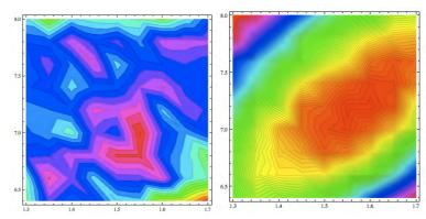
Fig. 19.45 a. Transmission map (red is high). The optimum transmission is obtained at alpha = 1.55, beta-7. Contour range is 69.5%-71.5% transmission b. Objective function map. The minimum is at alpha = 1.56 beta = 7.2. Objective function contour range is equivalent to 87.7%-91.7% transmission.
