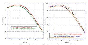
Fig. 14.8 Left - Demonstration of how the choice of radial mesh size can influence transmission. Right - Equivalent r-mesh extents for *BEAMPATH RZ* and *pteqHI schefftm*.
