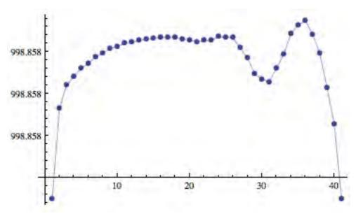
Fig. 19.7 Potential on the axis for on-axis beam, for Poisson cycle variables m=10, n1 = n2 = 14. The difference between the maximum and minimum is  $4.3 \times 10^{-8}$ %.
