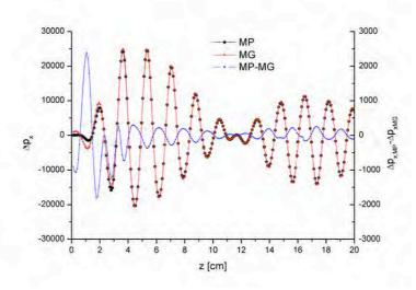
Fig. 17.42 Transverse kicks from multipole expansion method and multigrid Poisson solver on a certain particle along the beginning of the RFQ.
