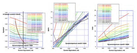
Fig. 19.36. a,b,c. Emittance (dynamic aperture), alpha and beta of the ellipse fitted to the rms dynamic aperture, vs. beam current, for the 16 RFQs set 'new 20110826'.
