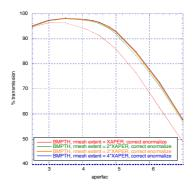
Fig. 14.6 Transmission curves for different BEAMPATH RZ space charge radial mesh boundaries.
