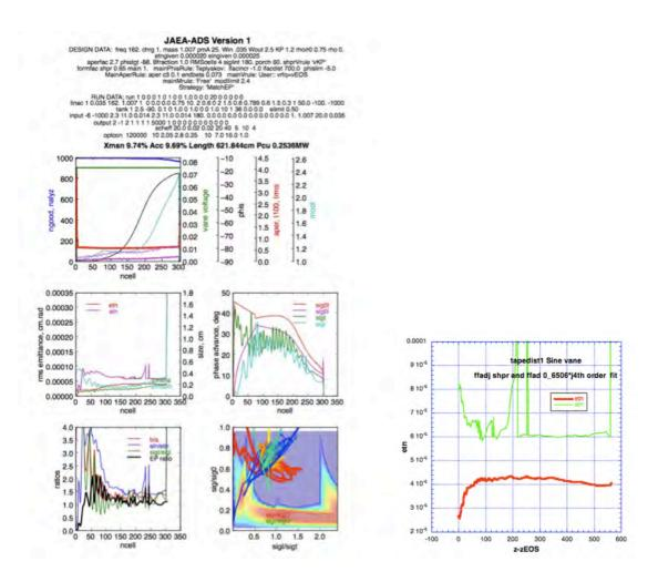
Fig. 28.5. Sine vanes. ffadj =  $0.6506*(4^{th} \text{ order polynomial fit}) \sim (b/a)_{experimental})/(b/a)_{design} = (b/a)_{experimental})/1.25 = ~1 -> adjusted ~ design bunch. Length 621 cm - same as base design...$
