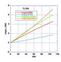
Fig. 27.23. Number of cycles of various phase advances over ACS length:  $s0t: 5.926, \quad st: 4.5756, \quad sz: 1.7276, \\ sigpt: 5.9607, sigpl: 7.2213, \\ where sigp\_ are the plasma oscillation phase advances.$
