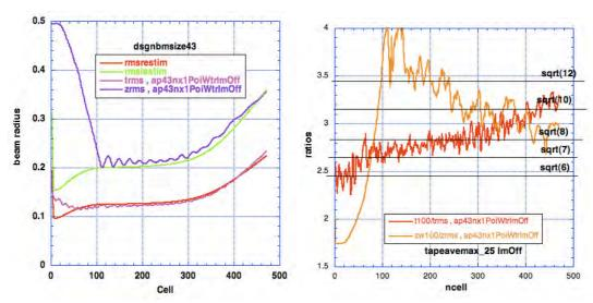
Fig. 22.14. Case1(43) Full Poisson simulation results but with space charge transverse boundary a cylindrical pipe with radius twice the maximum vane radius of the local cell, corresponding to Fig. 12.
