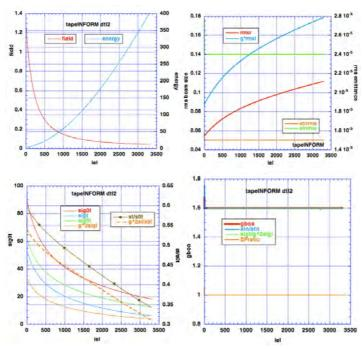
Fig. 27.1. Design performance of dtl2. (field is quadrupole fields, g = gamma,  $rmsr = a = trms = transverse rms beam radius, <math>g*rmsl = gbrms = \gamma*longitudinal rms beam size, sig = s = phase advance (s0 with zero current, s alone with beam current), t is transverse, l is longitudinal, n stands for normalized). The necessary growth in transverse beam size is seen at top right. No emittance growth. The EP condition = 1, with EP ratios = 1.6.$
