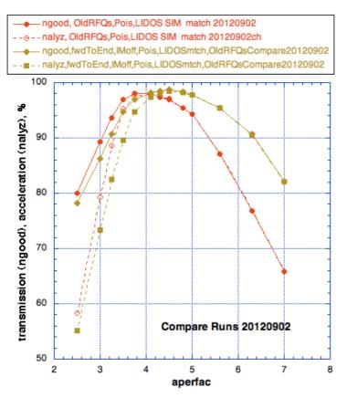
Fig. 19.50 Final result 2012 for the *aperfac* family, with full Poisson vane geometry for both external and space charge fields (red), and with full Poisson vane geometry for external field but a cylinder boundary for the space charge field (ochre). The shift in optimum EOS aperture is apparent.
