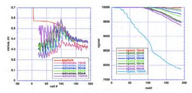
Fig. 21.12. Left: RFQ aperture and maximum particle radius as function of input beam current. Right: transmitted beam as function of input beam current.
