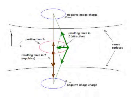
Fig. 16.12 Schematic of image forces acting in the RFQ.
