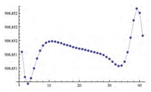
Fig. 19.5 Potential on the axis for on-axis beam, for Poisson cycle variables the standard m=5, n1 = n2 = 7. The difference between the maximum and minimum is 0.00011%.
