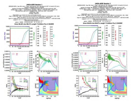
Fig. 29.3 Left – conventional 2-term vane profile, no truncation. Right – 2-term vane profile truncated at 0.5
