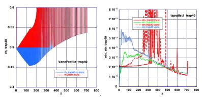
Fig. 29.22 Characteristics of trapezoidal vane modulation. There are heavy beam losses from z=~350.
