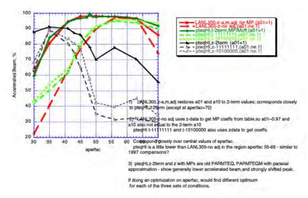
Fig. 13.2 Percent of accelerated beam using different simulation codes on the *aperfac* family of RFQs. This is a very early comparison in 2007. Other codes were also tested and gave other different curves, but were not discussable so are not shown. The general pattern of disagreement is what is important. here; the legend gives some details, e.g. the 8-figure numerical sequences show the multipole terms turned on (1) or off(0).
