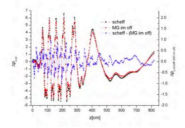
Fig. 17.49 Longitudinal space charge kicks from scheff and multigrid Poisson solver
