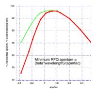
Fig. 13.1 Typical simulation result for the percentage of transmitted (green) and accelerated (red) beam for an *aperfac* family of 13 RFQs designed by changing one parameter.
