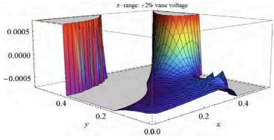
Fig. 17.32 Absolute difference of the potentials from the multipole expansion method and from the multigrid Poisson solver at the center of cell 150.
