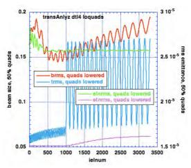
Fig. 27.12. dtl4 with quad reduction to 50%.
