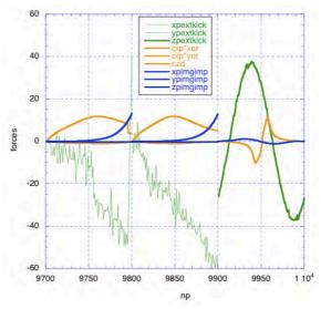
Fig. 16.13 Forces acting on test particles over one transverse focusing period (2 cells). Particles 9701-9800 are on x-axis, 9801-9900 on y-axis, 9901-10000 on z-axiz.
