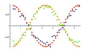
Fig. 19.39 X (blue) and y (green) are the variation of beam size from the average design value, of beam slices located in the  $2^{\circ}$ ,  $\beta\lambda/180$  region just after the end of the RMS, for 20 steps per cell. The input beam  $\alpha$  and  $\beta$  are for the best transmission match. Red and yellow are the x and y beam sizes from Eq.(1) (which does not include space charge effect) evaluated at the end of the RMS.
