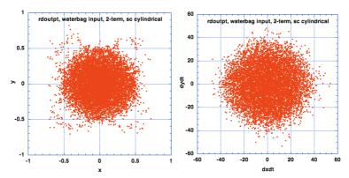
Fig. 22.4.b. Typical phase space distributions in an RFQ with 2-term external and cylindrically symmetric space charge fields.
