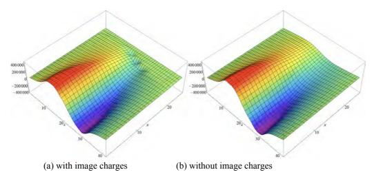
Fig. 17.53 Longitudinal field Ez from space charge at a xz-plane with and without image charges.
