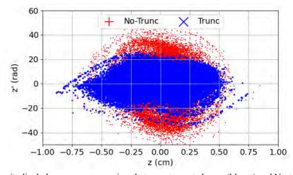
Fig. 29.24 Longitudinal phase space comparison between truncated vane (blue x) and No-truncated (red plus) at the end of the shaper, cell 165.
