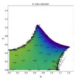
Fig. 17.39 Relative difference (MG-MP)/MG of absolute value of the electric field (E) in the xy-plane at the end of a accelerating cell.
