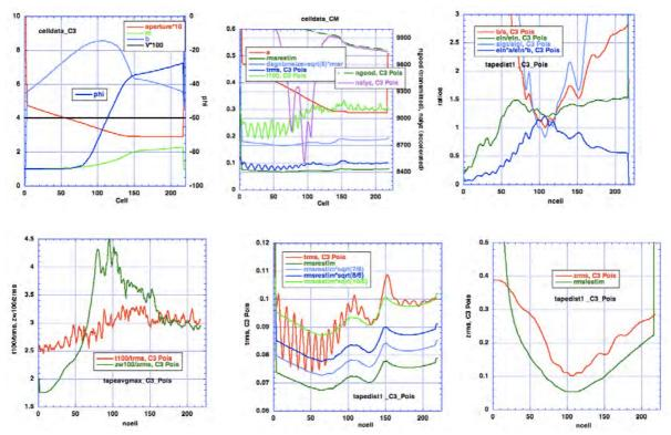
(NOTE!! – THIS RFQ IS NOT EP AT EOS!!) Constant aperture at end. Not EP, except briefly at cells ~100-120, but also evidence of 1:1 resonance cell 80-100, where scraping starts, then both losses -> Case 2(70). Trms redistribution – immediately to ~parabolic, then to Gaussian; no redistribution at low current. Like C1 and IMP\_ADS.
