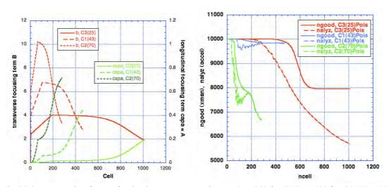
Fig. 22.9. a. Focusing factors for the three cases. Maximum s0t = 23° for C3(25), 42° for C1(43), 59° for C2(70). b. Transmission (ngood) and accelerated (nalyz) particles from 10000 particle waterbag input distribution.
