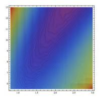
Fig. 19.41 Contour map of the phase wobble objective function as function of the input match  $\alpha$  (abcissa) and  $\beta$  (ordinate). Red is high, violet is small.
