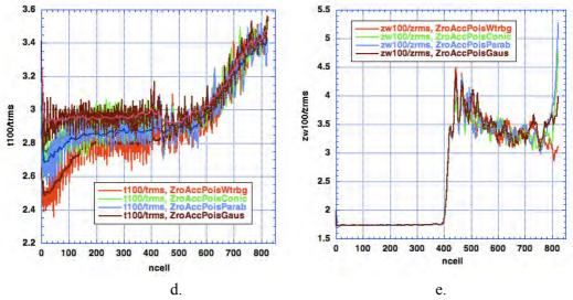
Fig. 22.2. a.) Ratio of 100% transverse beam size to the transverse rms beam size (t100/trms) b.) corresponding longitudinal ratio (zw100/zrms).
