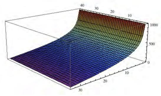
Fig. 19.3 Space charge x vs. z potential of on-axis beam.
