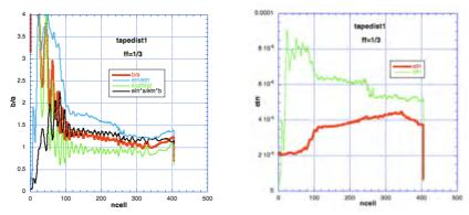
Fig 28.2. 2term vanes. Form factor set to 1/3; EP conditions and rms emittances. There is no saturation of either the modulation or synchronous phase. The total length in increased to 735 cm.
