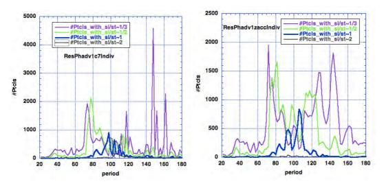
Fig 21.9. Number of particles within  $\pm 0.03$  band of  $\sigma^l/\sigma^t = 0.33$ , 0.5, 1.0 and 2.0 resonances. Left – particles being transmitted at each period. Right – particles accelerated successfully to the end of the RFQ.
