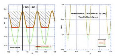
Fig. 29.21 shows the typical truncation, for z 100-105 (left) and z 400-420 (right).
