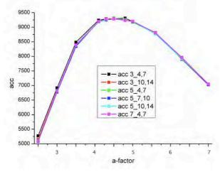
Fig, 17.21. External field grid: Influence of the number of multigrid iterations (first number) and smoothing cycles (second number and third for ratios of hx/dz greater than 4) on the number of accelerated particles.
