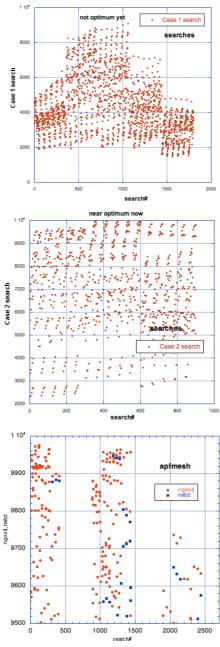
Fig. 9.1 Results of three successive searches over the six parameters of Eqn.(1). The vertical axis is the number of particles transmitted (ngood – red) and the number of particles accelerated to within 3% of the final synchronous energy (nalyz – blue).
