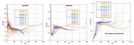
Fig. 13A1.8. The first three rows show the rms beam sizes, rms normalized emittances, the rms phase advances per  $\beta\lambda$ , and the associated equipartitioning ratios. The fourth row shows the transverse and longitudinal tune depressions and the equipartitioning (EP) condition. Only the RFQs near the optimum of Fig. 1 can actually attain the EP condition throughout the RFQ.
