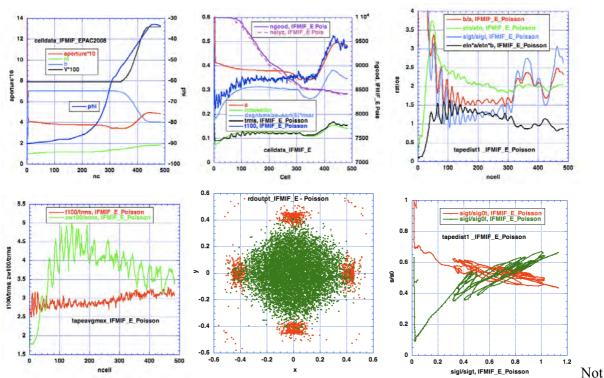
EP, continuous both losses - Case 3(25). No trms redistribution. Particles riding beside vane tip. Parameters  $\sim$ flat at end.
