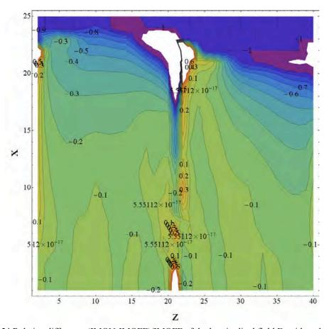
Fig. 17.54 Relative difference (IMON-IMOFF)/IMOFF of the longitudinal field Ez with and without image charges in the xz-plane.
