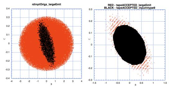
Fig.19.31a. Typical pattern. Red - normal Type 6 input beam, alpha=0, emittance and beta large enough to encompass all the accepted particles. Black – accepted particles. Fig. 19.31b Comparison of transverse acceptance:for particles all injected at synchronous phase and energy
