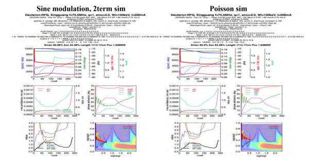
Fig. 25.1. *LINACSrfqSIM* of Xingguang Design. Sinusoidal vane modulation. Left - 2term simulation, right - Poisson simulation. (Title showing I=200mA is a title only – DESIGN DATA and RUNDATA show designed and run at 400 pmA.)
