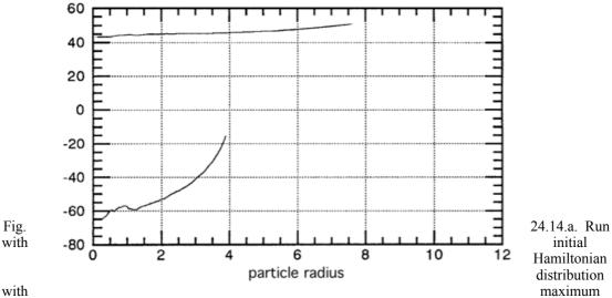
radius = 5,  $\mu$  = 0.84. A mismatch of 1.5 increases the maximum radius to 7.5. Instantaneous phase advance vs. radius for all particles; upper curve is at a central density minimum near the beginning of the run, lower curve is at an adjacent central density peak.
