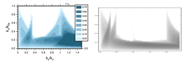
Fig. 1.3. Hofmann Chart (left) for longitudinal-to-transverse emittance ratio eln/etn = 2.0; thus kz/kx = 0.5 is the equipartitioned condition for this chart. (right) for eln/etn = 1.03. The shading represents a growth rate. The values are for a special case and should be ignored. The curious lack of response on one side of resonances is commented by Hofmann in Sec.21.6, where it it shown that there is actually a reaction on both sides.
