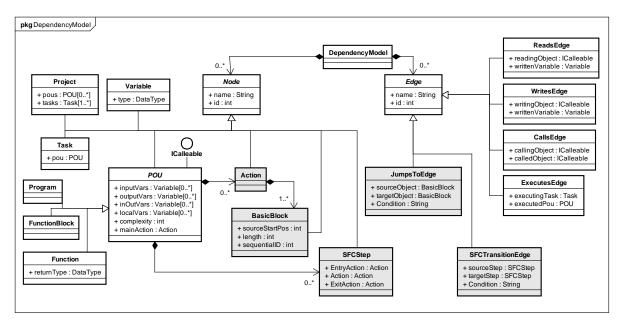
Figure 2: Extended (grey shaded) dependency model for IEC 61131-3 based on (Feldmann et al., 2016) for code analysis
