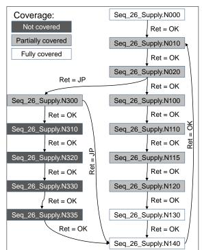
Figure 9: Coverage assessment unveils untested fault handling routine: The code branch for documenting faulty cycle timing was never executed during the tests
