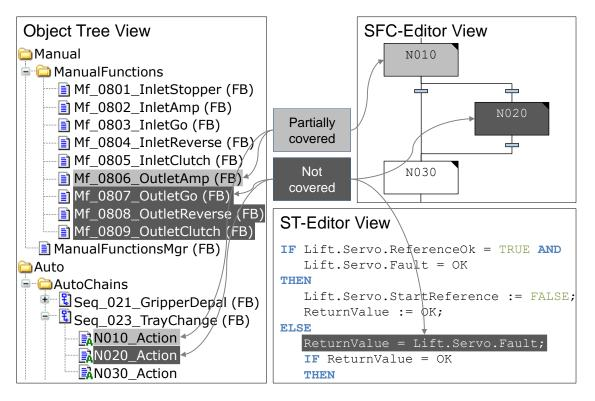
Figure 7: Mock-up of editor integration of coverage visualization: Insufficiently covered items can be easily spotted, such as POUs in the object tree view (left), steps in the SFC-editor view (upper right) and basic blocks in the ST-editor view (lower right)
