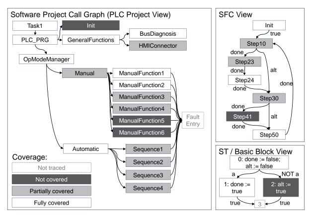
Figure 6: Hierarchical coverage views as developed for the approach: A software project call graph (left) gives a quick overview of covered (light grey and white) and uncovered (dark grey) POUs. More detailed views can unveil uncovered parts of the code from SFC level (upper right) to ST level (lower right).
