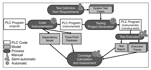
Figure 1: Concept overview of coverage assessment for aPS software: An original PLC program is automatically instrumented and extended by executable test cases. After semi-automatic system test execution, execution traces, a dependency model and information about generated trace points are used to automatically calculate test coverage, which supports testers in adequacy assessment.
