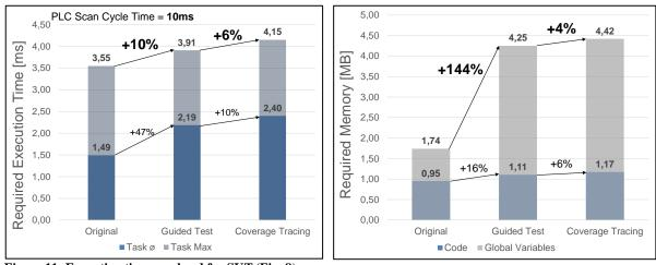
Figure 11: Execution time overhead for SUT (Fig. 8) Figure
