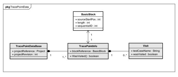
Figure 4: Trace point database: Meta model to store information about instrumented points in the code and later relation to test case execution traces represented as "visits" or the respective trace point.
