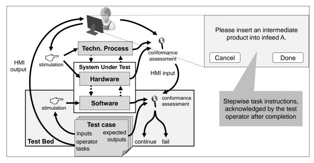
**Figure 5: Inclusion of the tester (engineer or technician) into the system testing process** (Ulewicz & Vogel-Heuser, 2016): **By showing step-wise testing instructions on a display, the human can stimulate and check the system wherever the test bed cannot (hardware and technical process)**
