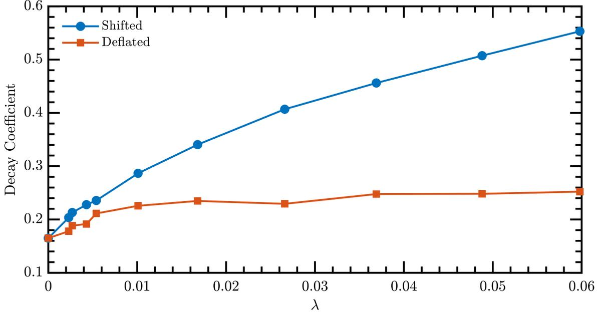
**Figure 1.** The decay coefficient extracted from  $(D + \lambda I)^{-1}$  and  $(I - P(\lambda))D^{-1}$ , where  $P(\lambda)$  is the projector to the low singular space that includes all singular triplets up to  $\lambda$ .
