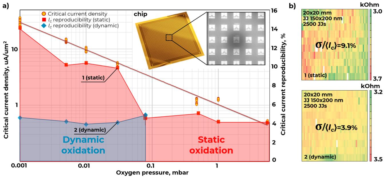
**Figure 3.** Critical current density and critical current reproducibility of the Al/AIO<sub>x</sub>/Al junctions vs oxidation method and oxygen pressure (a); critical current variation ( $\sigma/I_c$ ) of JJs for static and dynamic oxidation (b).
