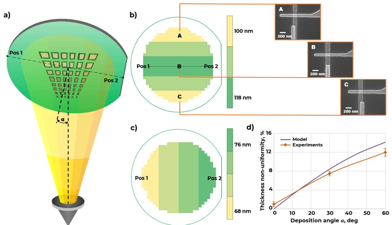
**Figure 1.** Thin film evaporation diagram from crucible at an angle to a substrate (a); distribution map of JJ dimensions over a 4" wafer ( $\alpha = 0^\circ$ ) (b); distribution map of the film thickness over a 4" wafer ( $\alpha = 60^\circ$ ) (c); the dependence of a film thickness nonuniformity vs deposition angle  $\alpha$  (d).
