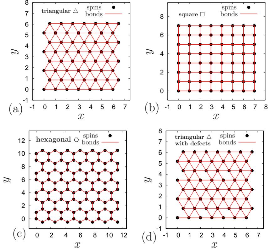
FIG. 2. Decorations of lattices: (a) regular triangular lattice ( $\Delta$ ) of size  $7 \times 8$ , *i.e.*,  $N = 56$ ; (b) regular square lattice ( $\square$ ) of size  $8 \times 8$ , *i.e.*,  $N = 64$ ; (c) regular hexagonal lattice ( $\circ$ ) of size  $14 \times 8$ , *i.e.*,  $N = 112$ ; (d) triangular lattice ( $\Delta$ ) with 12 defects of type  $b = 5$  (*i.e.*, 6 missing bonds) of size  $7 \times 8$ , *i.e.*,  $N = 56$ .
