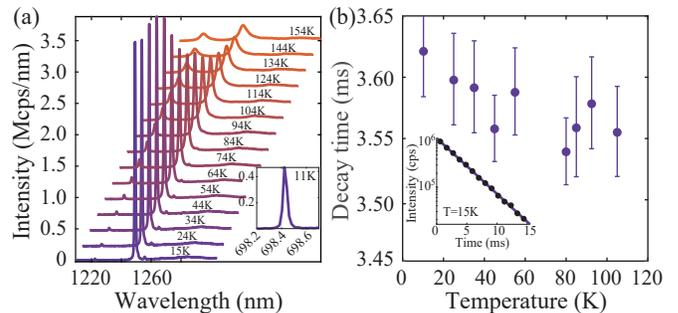
FIG. 5. Optical spectroscopy of  $\text{Ni}^{2+}:\text{MgO}$ . (a) Temperature dependence of the emission spectrum. The inset (using the same units as in the main figure) shows the  $\text{Cr}^{3+}$  line around 698 nm. (b) Fluorescence decay-time versus temperature. The inset presents a characteristic fluorescence decay curve (semi-logarithmic scale).
