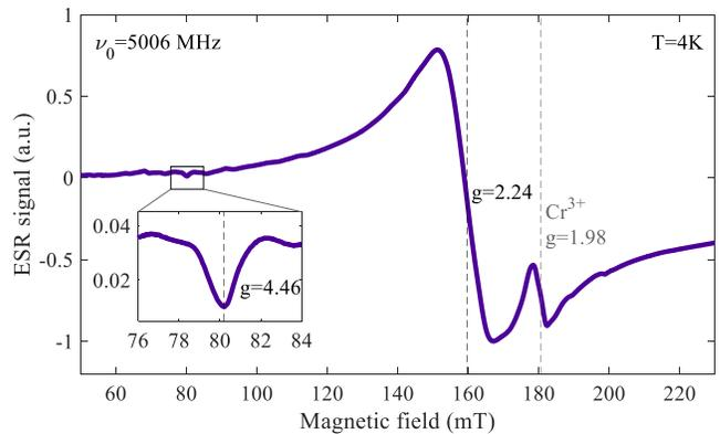
FIG. 2. Electron spin resonance (ESR) spectrum of the ground-state spin of  $\text{Ni}^{2+}:\text{MgO}$ . The magnetic field was calibrated using the  $\text{Cr}^{3+}$  line at  $g = 1.98$ . The inset magnifies the spectrum around the  $\Delta m_s = 2$  transition.
