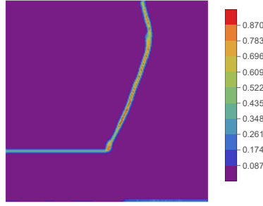
Figure 27: Kalthoff-Winkler test v_y = 20 m/s: tensile fractures.
