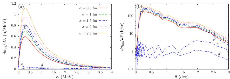
**Fig. 2** Breakup cross section of  $^{19}\text{C}$  on  $^{208}\text{Pb}$  at 67A MeV (a) plotted as a function of the  $^{18}\text{C}$ -n relative energy  $E$  after dissociation, and (b) plotted as a function of the scattering angle of the  $^{18}\text{C}$ -n centre of mass for energies  $0 \leq E \leq 0.5$  MeV. In both cases,  $s$ ,  $p$ , and  $d$  components are shown separately for the  $\sigma = 1.5$  fm case (blue dash-dotted lines).
