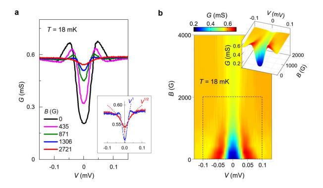
Figure 3| Magnetic field-driven phase transition. a, The tunnelling conductance G(V, T = 18 mK) with increasing magnetic field. The inset shows an enlarged view of the G(V) curves measured at B = 1306 and 2721 Gauss. The broken dotted lines are fitted to the curves using |V| and  $|V|^{1/2}$  relations. b. Intensity map of the *B*-dependent G(V) at T = 18 mK. The inset shows the three-dimensional enlarged view of the *B*-dependent G(V) curves in the low *B* region.
