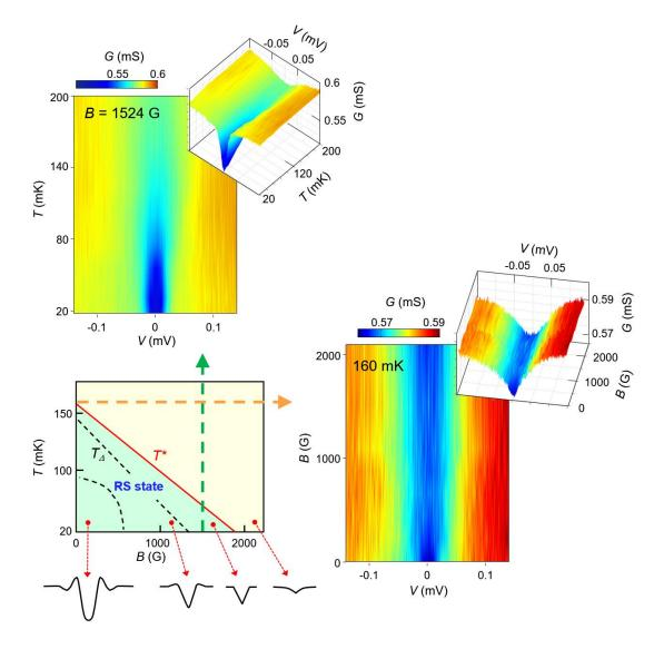
**Figure S2.** Intensity maps of the G(V) curves showing the evolution of the ZBA spectrum and the V-groove spectrum along the different path in the *T-B* phase diagram.
